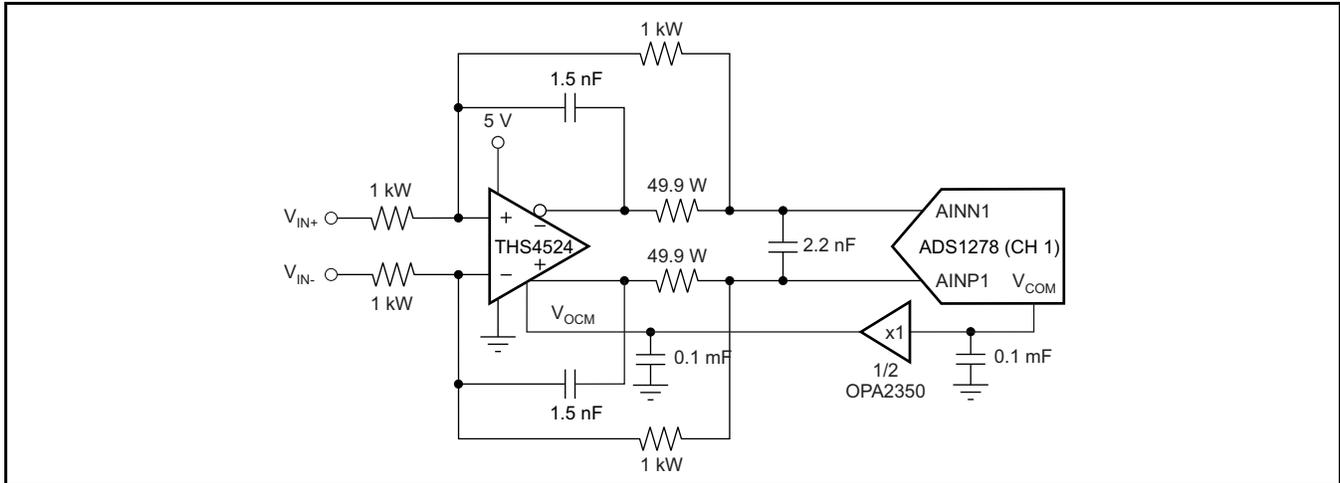
Figure 82. THS4524 and ADS1278 (Ch 1) Test Circuit
