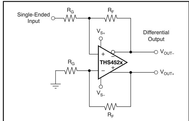
**Figure 62. Single-Ended Input to Differential Output Amplifier**
