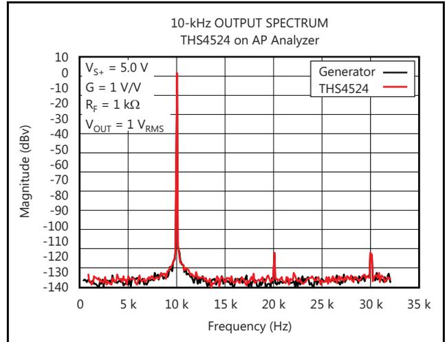
Figure 71. THS4524 1- $V_{RMS}$  10-kHz FFT Plot
