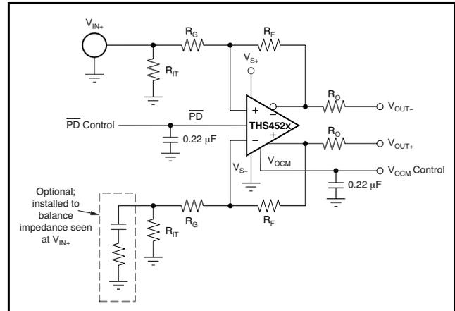
Figure 64. THS4524 DC-Coupled Single-Supply with Single-Ended Inputs
