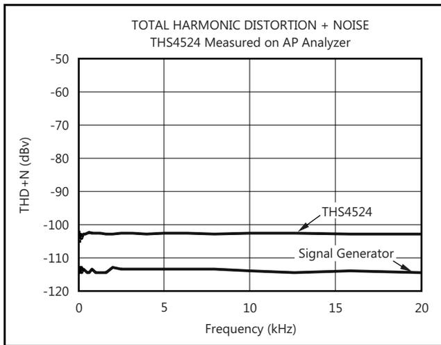
Figure 70. THS4524 1- $V_{RMS}$  20-Hz to 20-kHz THD+N
