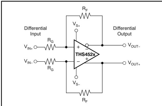
**Figure 61. Differential Input to Differential Output Amplifier**
