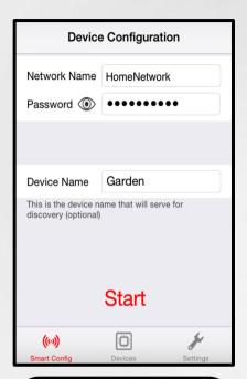
Smart Config provides an extremely simple way to add new devices to Wifi router. It is as simple as entering the password and an optional name and clicking Start.
