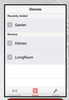
Devices advertise their presence through mDNS. Clicking on the name of the device will open the device's website, which will enable you to configure optional settings
