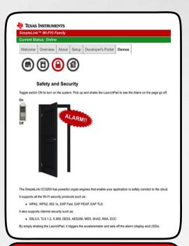
**Sensor Example:** Uses the accelerometer to display an alarm on the web page and flash LEDs
