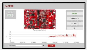
Displays temperature data that has been sent by the CC3200. Remote control an LED from the web page
