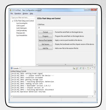
Console outputs information requesting input and debug information that can be used to solve problems
