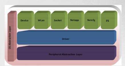
TI SimpleLink Framework provides a wide set of capabilities ranging from basic device management through wireless network configuration, BSD socket services and more. These capabilities are segregated into individual modules. Each module represents different functionality capability of the SimpleLink Framework.
