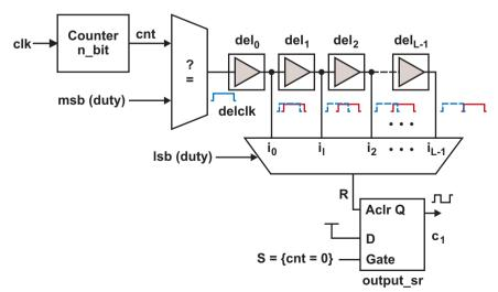
Fig. 22. Hybrid DPWM with external clock.
