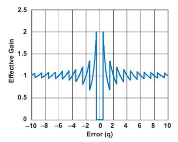
b. ADC gain due to quantization.
