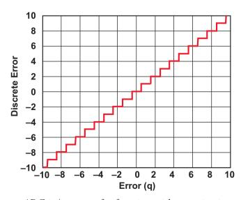
a. ADC in/out transfer function with quantization.
