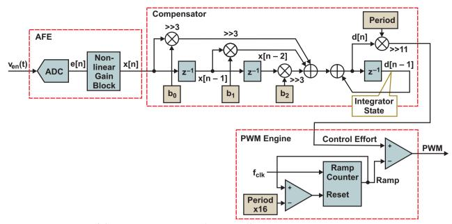
Fig. 24. Location of the integrator state in the controller system.
