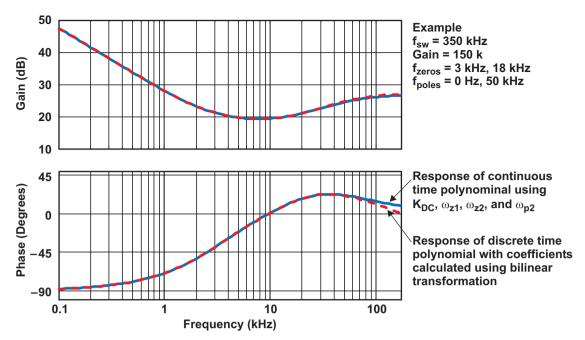
Fig. 12. Frequency response of continuous-time and discrete-time compensator.
