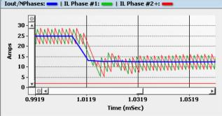
Fig. 35. Simulation results of a 50- to 25-A load transient for a synchronous two-phase buck converter.
