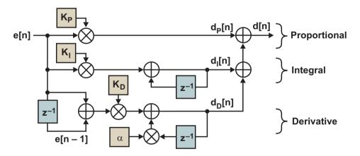
Fig. 11. PID digital-filter implementation.
