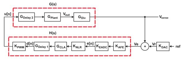
Fig. 3. Closed-loop block diagram.
