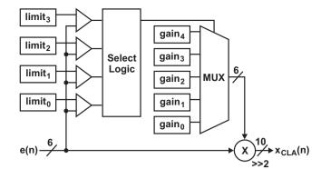
Fig. 19. Digital controller with nonlinear quantization.
