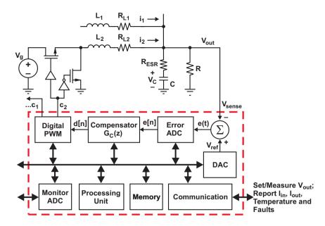
Fig. 2. Digital controller in an SMPS.
