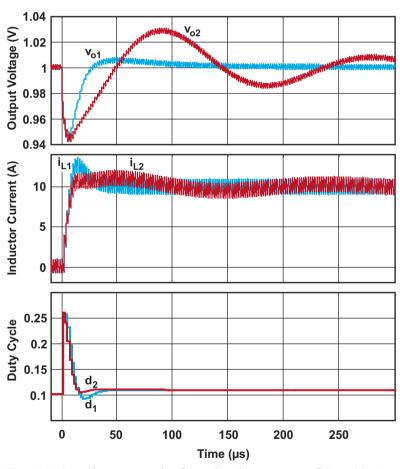
Fig. 15. Simulation results for a load transient of 1 to 10 A.
