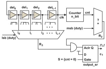
Fig. 23. Hybrid DPWM with ring oscillator.
