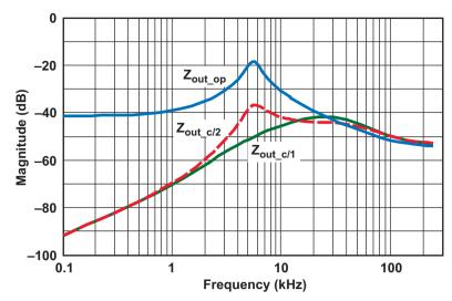
Fig. 14. The magnitude response of the open-loop and closed-loop output impedance.
