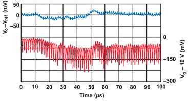
Fig. 37. The step-up load-transient response.
