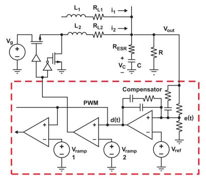
Fig. 1. Analog-controlled SMPS.
