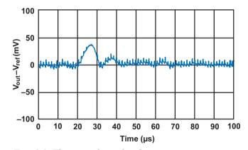
Fig. 36. The step-down load-transient response.
