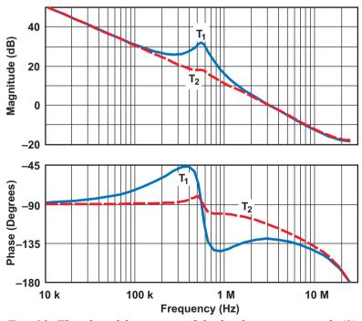
Fig. 13. The closed-loop gain of the buck converter with (1) real zeros and (2) complex zeros.
