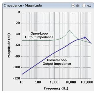
Fig. 33. Frequency response of open-loop and closed-loop output impedance.
