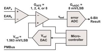
Fig. 17. Block diagram of an eADC together with a programmable DAC.
