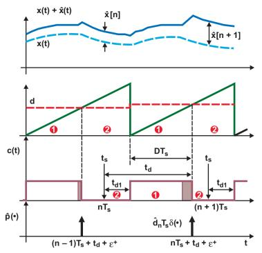
Fig. 6. Waveforms illustrating derivation of a discretetime model for a digitally-controlled SMPS.
