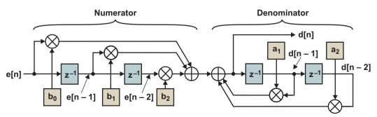
Fig. 10. Direct-form digital-filter implementation.
