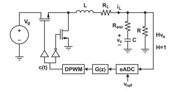
Fig. 5. Voltage-mode, closed-loop buck converter.
