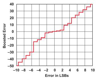
a. Transfer function after nonlinear gain. Fig. 20. Application of nonlinear gain.
