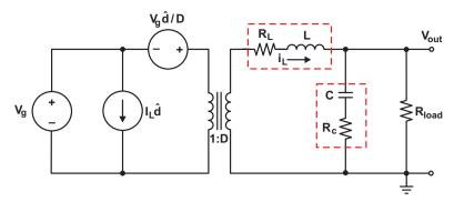
Fig. 4. Small-signal model of a buck converter with losses.
