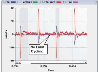
Fig. 25. Limit cycling with low nonlinear gain.
