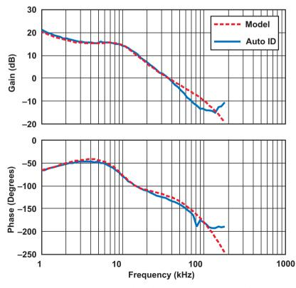
Fig. 27. Bode plot measured with Auto-ID versus model.
