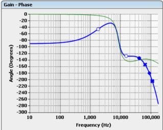
Fig. 32. Loop gain and control-to-output-voltage frequency response.
