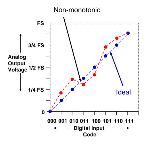
Non-monotonic DAC's are not appropriate for control loop Applications!
