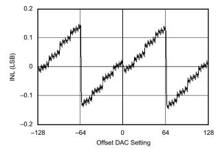
Figure 5. INL vs Offset DAC Setting
