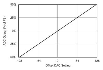
Figure 3. ADC Output vs Offset DAC Setting
