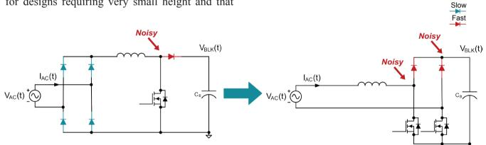
Figure 25 – Bridge vs bridgeless high dV/dt nodes.
