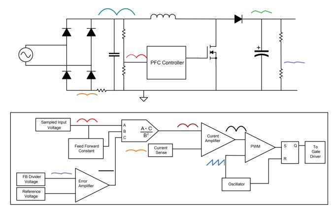
Figure 19 – CCM PFC block diagram using average current mode control.
