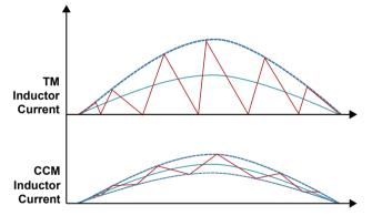
Figure 27 – CrCM/TM and CCM inductor ripple current comparison.
