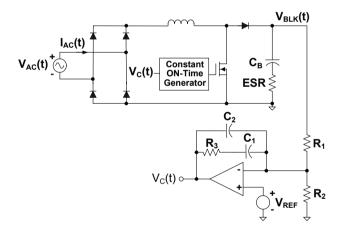
Figure 16 – PFC behavioral model and compensation.
