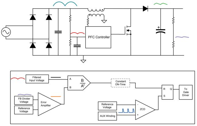
Figure 18 – CrCM PFC block diagram using constant on-time.
