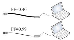
Figure 3 – Laptop cable comparison.
