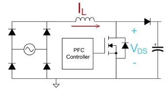
Figure 11 – Simplified boost PFC schematic.
