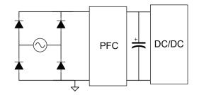
Figure 6 – Introduction of power factor correction stage.
