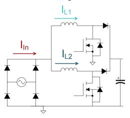
Figure 22 – Interleaved boost PFC.
