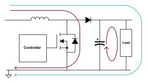
Figure 7 – Boost converter power paths.
