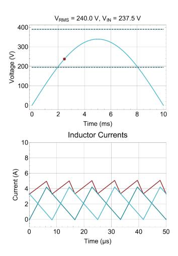
Figure 23 – Interleaved boost inductor currents and total input current ripple.
