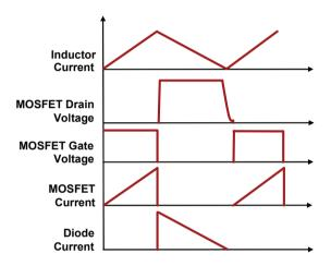
Figure 8 – Boost converter waveforms.
