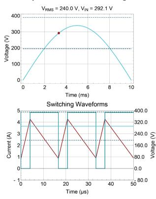
Figure 20 – Inductor current and MOSFET drain waveforms near peak of AC line.
