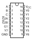
Figure 3-1. CD54AC138 J Package, CD74AC138 E or M Package (Top View)
