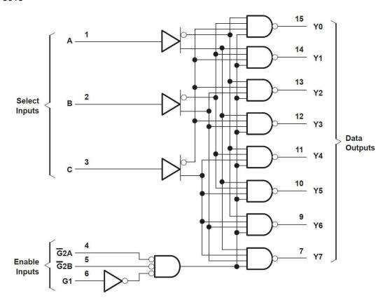
Logic Diagram (Positive Logic)
