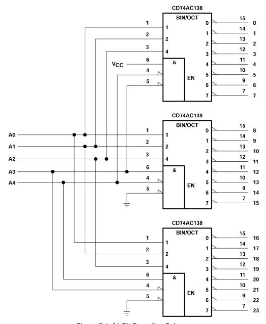
Figure 7-1. 24-Bit Decoding Scheme
