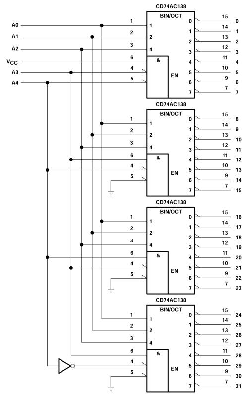
Figure 7-2. 32-Bit Decoding Scheme
