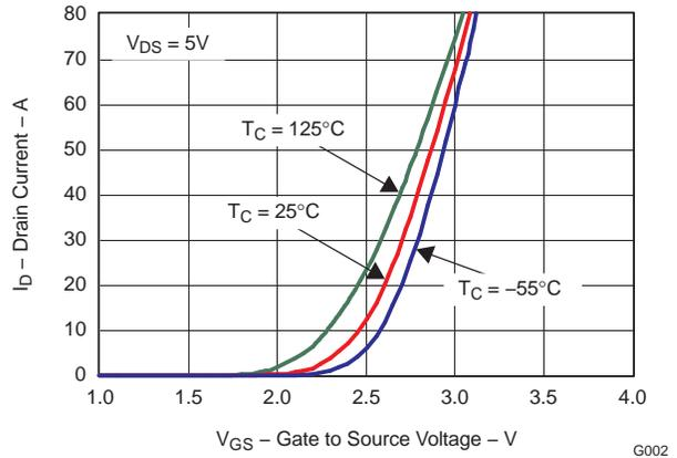
**Figure 3. Transfer Characteristics**
