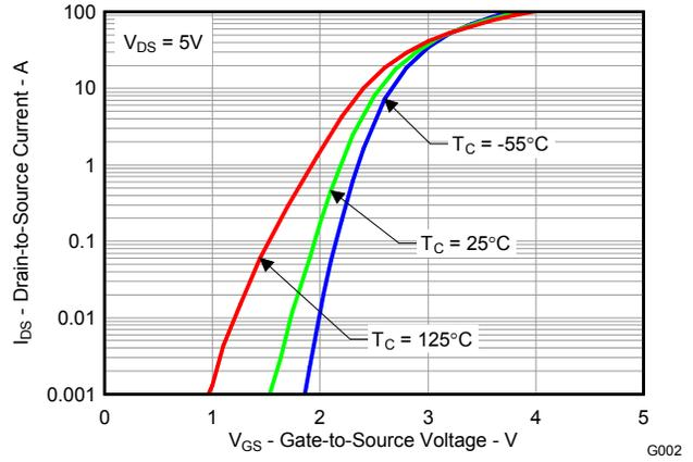
**Figure 3. Transfer Characteristics**
