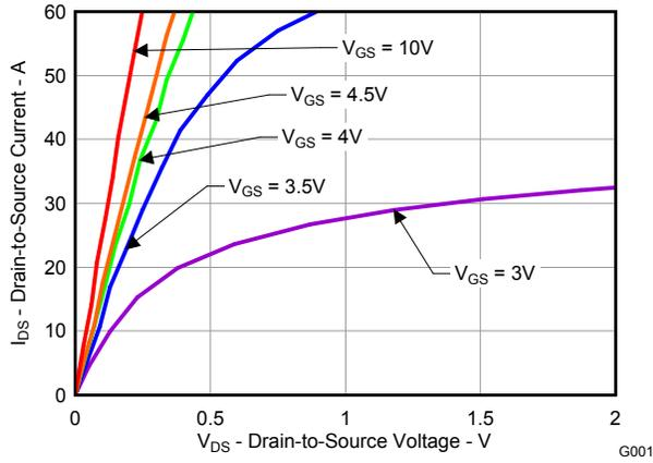
**Figure 2. Saturation Characteristics**
