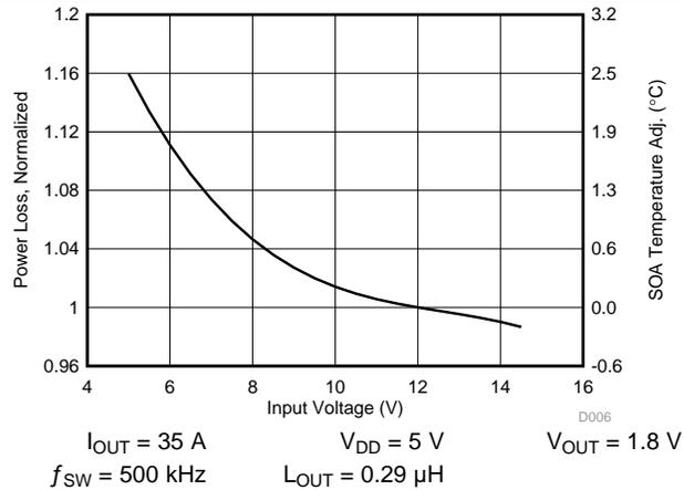
Figure 9. Normalized Power Loss vs Input Voltage
