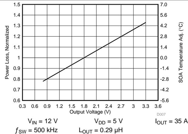
Figure 10. Normalized Power Loss vs Output Voltage
