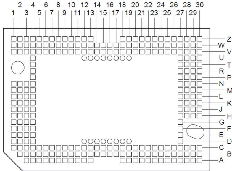
**Figure 5-1. FXK Package 257-Pin CLGA Bottom View**
