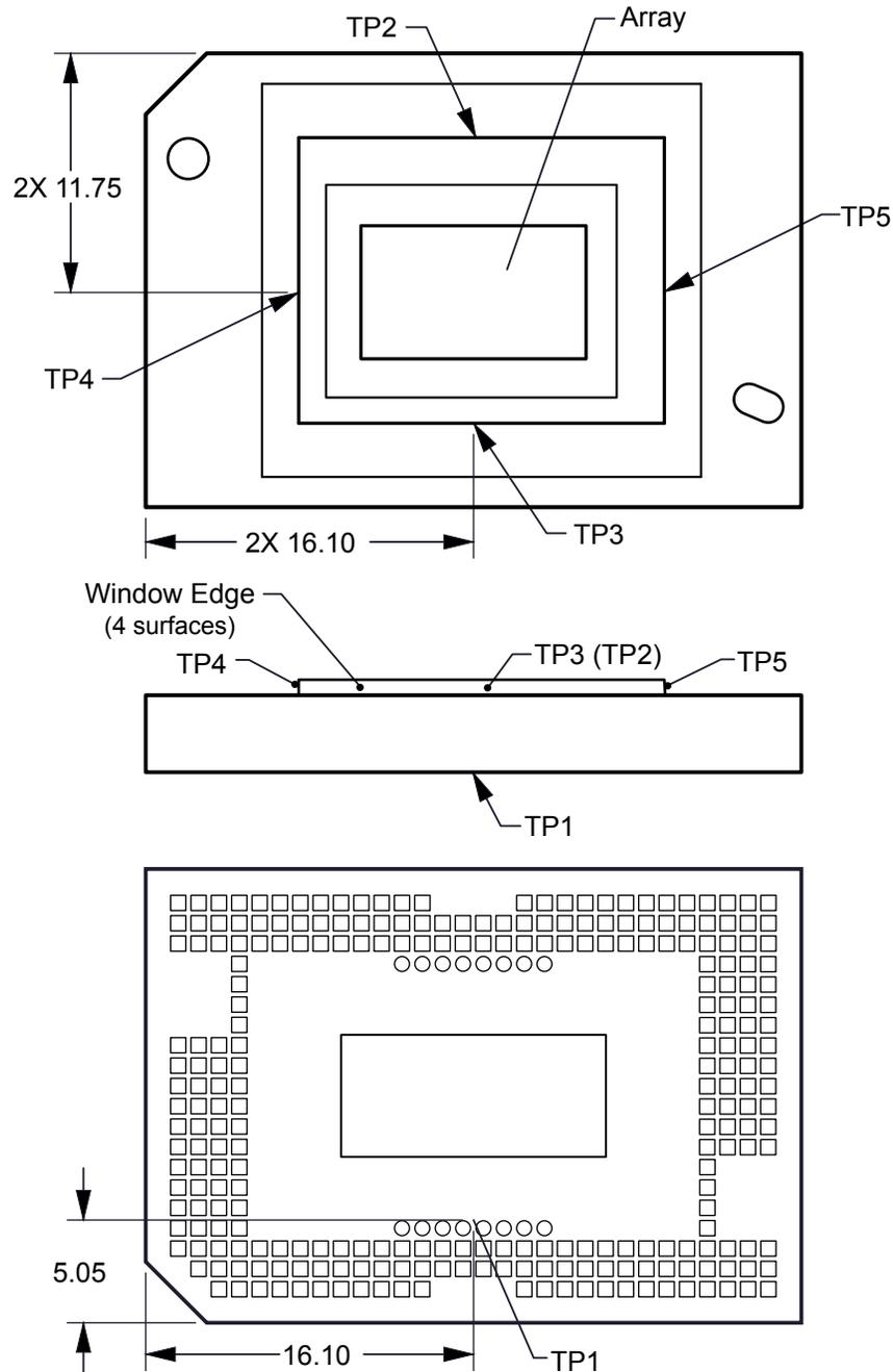
**Figure 7-2. DMD Thermal Test Points**
