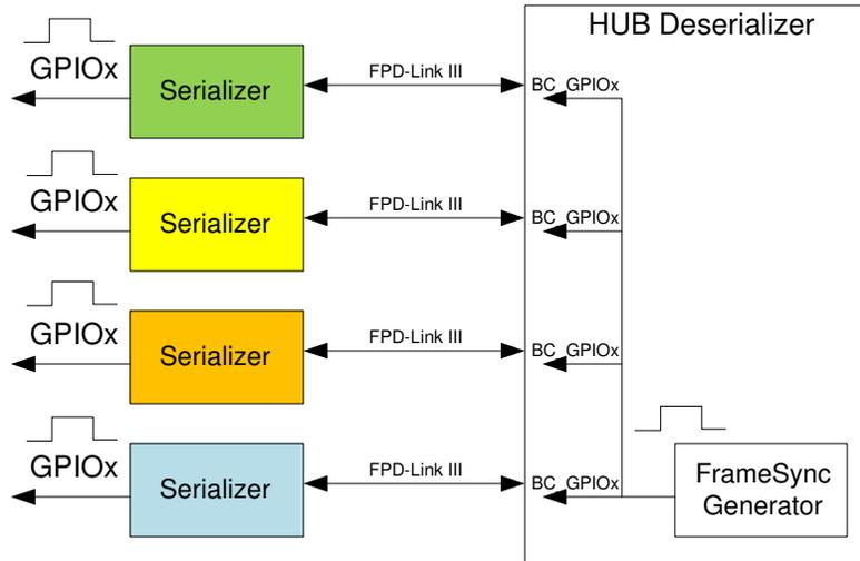
Figure 7-13. Internal FrameSync
