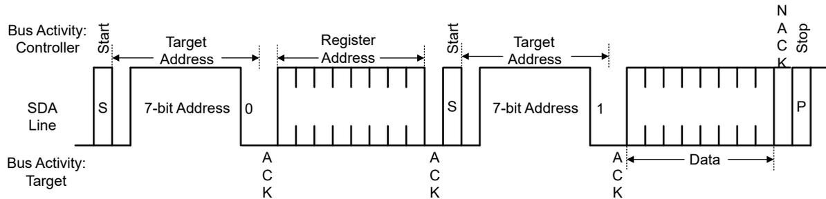
Figure 7-20. Serial Control Bus — READ
