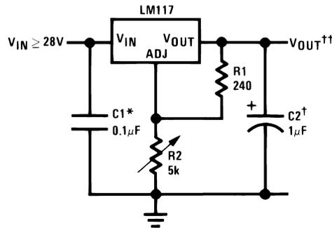
Full output current not available at high input-output voltages
