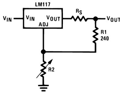
Figure 16. Regulator with Line Resistance in Output Lead
