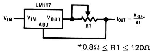
Figure 31. Precision Current Limiter
