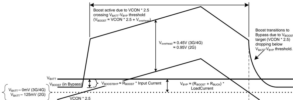
Figure 28. Boost Operation showing VCON- $V_{\text{BATT}}$  Relationship
