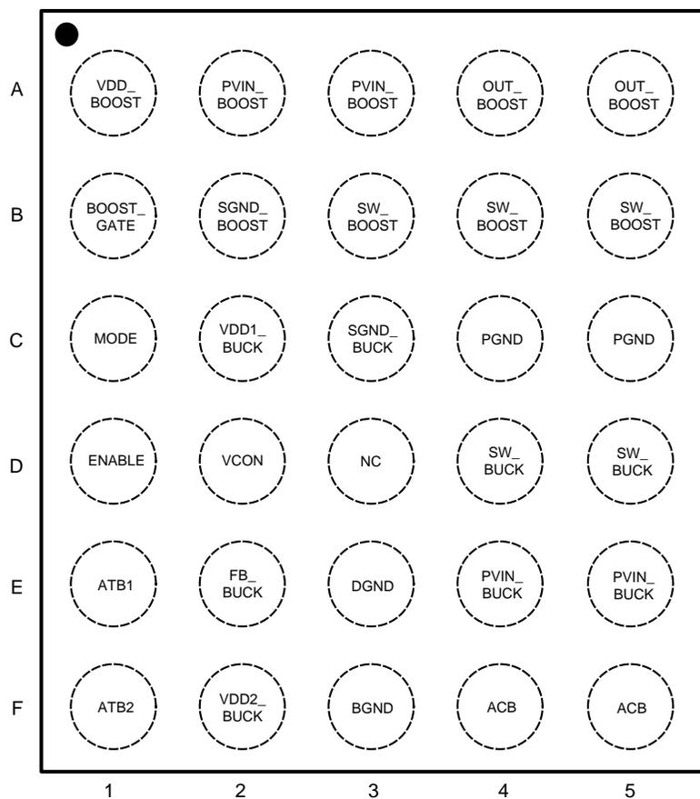
**Figure 1. 30-Bump Thin DSBGA Package (0.4 mm pitch)
