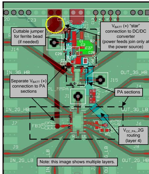
Figure 31. LM3248  $V_{BATT}$  Star Connection and  $V_{CC\_PA}$  Routing
