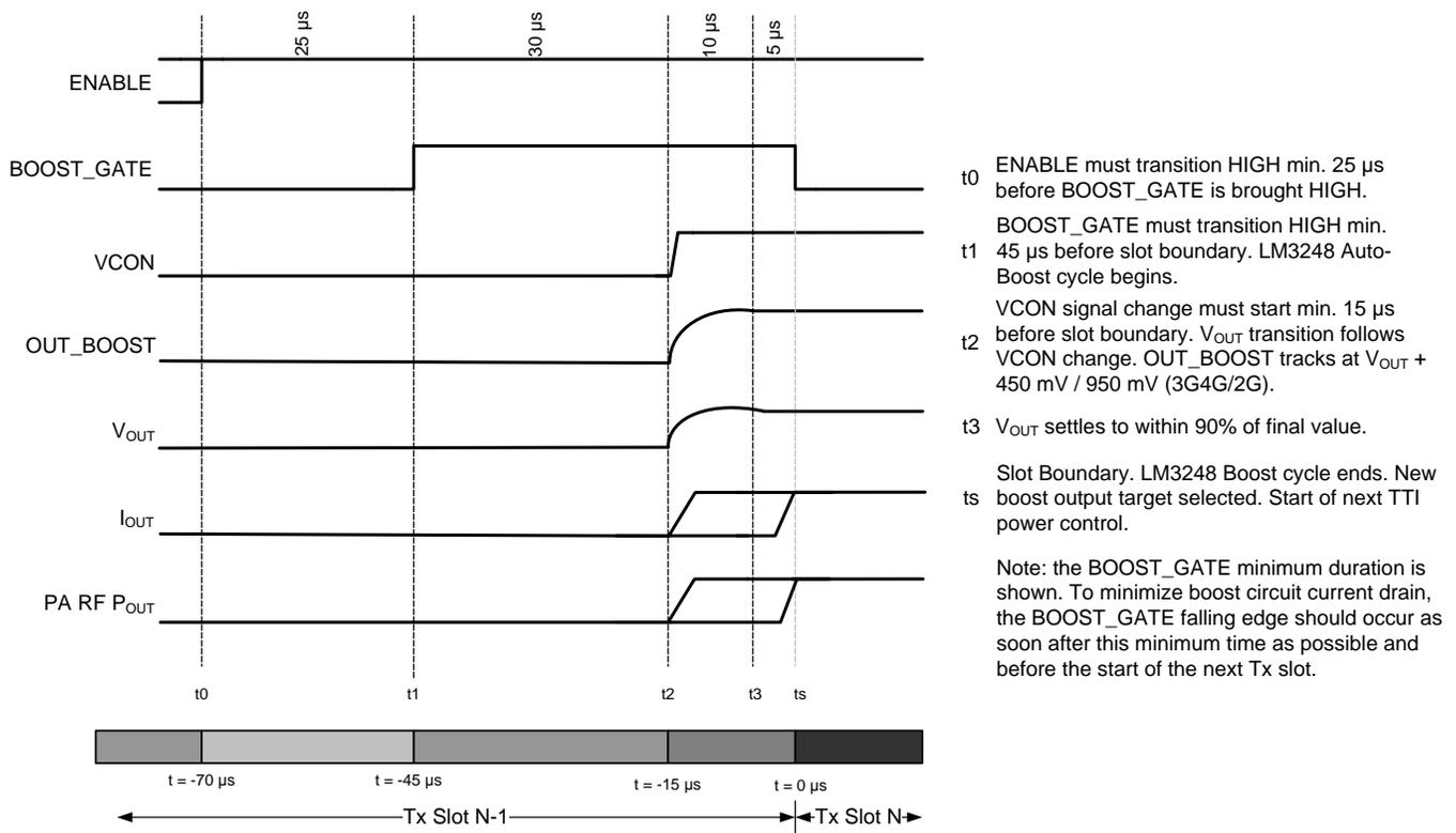
Figure 2. Startup + Optional Boost Timing Sequence
