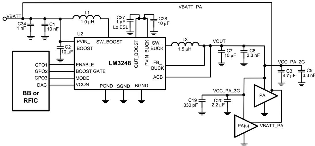
**Figure 29. Simplified LM3248 RF Evaluation Board Schematic**
