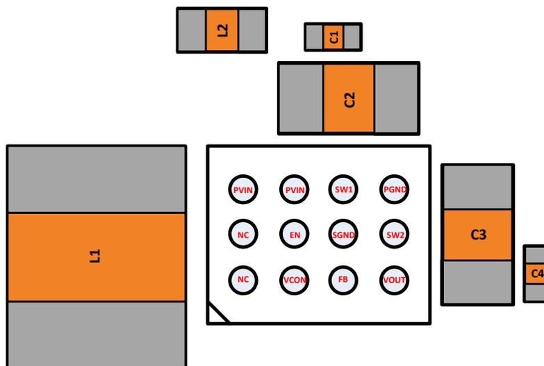
Figure 17. LM3269 Recommended Parts Placement (Top View)
