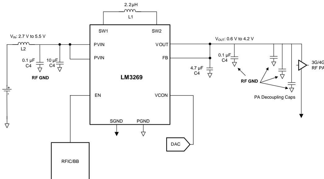
Figure 16. Simplified LM3269 RF Evaluation Board Schematic
