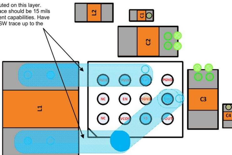
Figure 20. Board Layer 3 - SW Routing
