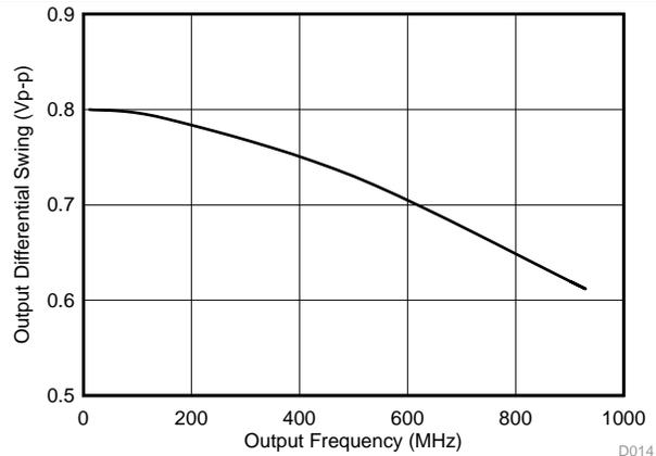
Figure 2. LVDS Differential Output Swing vs Frequency
