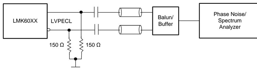
Figure 7. LVPECL Output AC Configuration During Device Test
