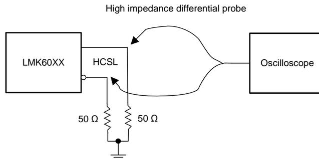
Figure 6. HCSL Output DC Configuration During Device Test
