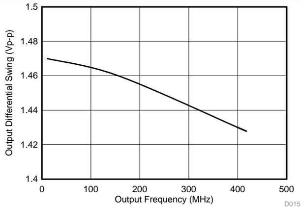
Figure 3. HCSL Differential Output Swing vs Frequency
