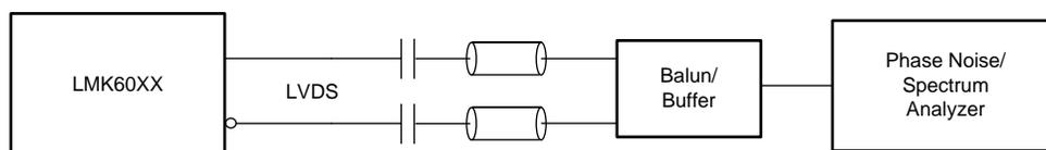
Figure 8. LVDS Output AC Configuration During Device Test
