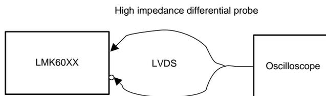
Figure 5. LVDS Output DC Configuration During Device Test
