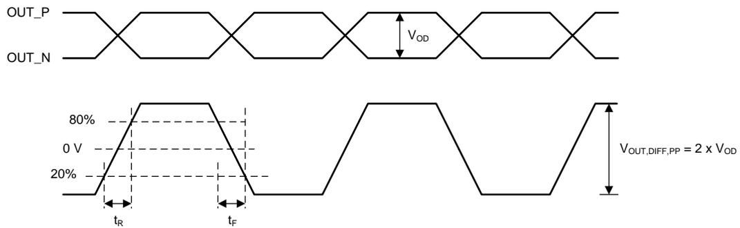
Figure 11. Differential Output Voltage and Rise/Fall Time
