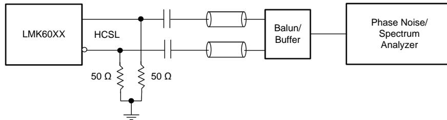
Figure 9. HCSL Output AC Configuration During Device Test
