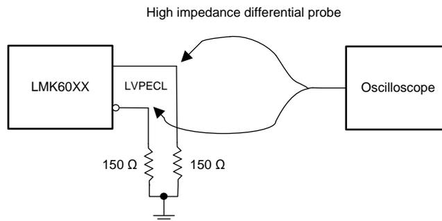
Figure 4. LVPECL Output DC Configuration During Device Test
