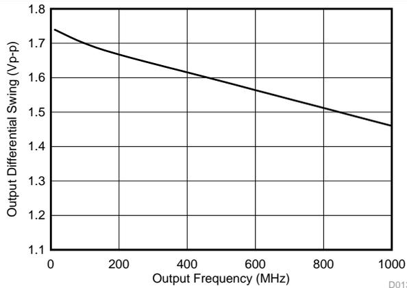
Figure 1. LVPECL Differential Output Swing vs Frequency
