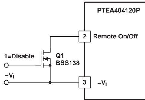
Figure 5. Recommended Control or Remote On/Off Input
