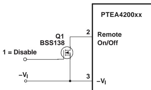
**Figure 9. Recommended Control or Remote On/Off Input**
