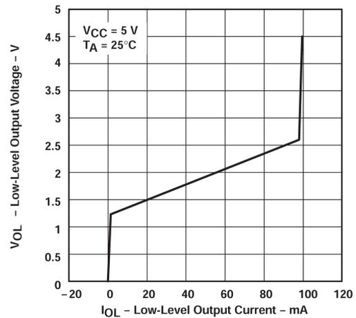
**Figure 5-2. Low-level Output Voltage vs Low-level Output Current**
