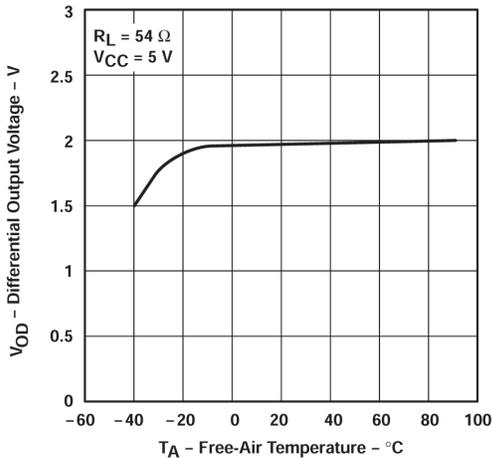
**Figure 5-3. Differential Output Voltage vs Free-air Temperature**
