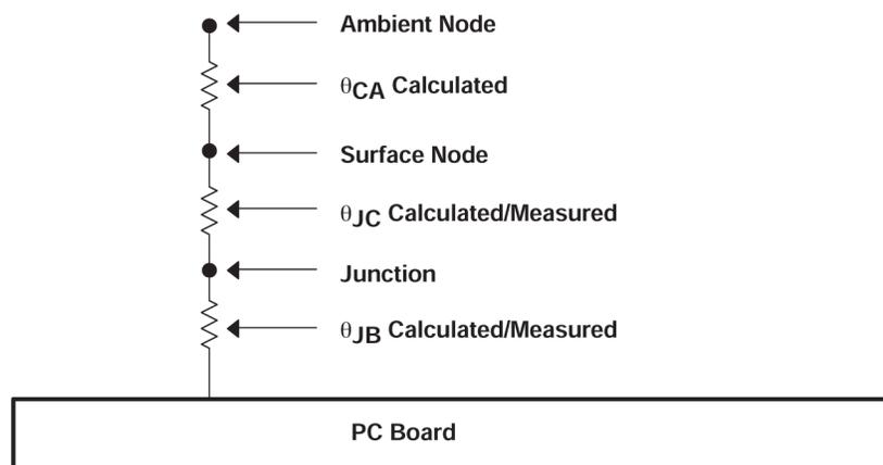
**Figure 7-1. Thermal Resistance**
