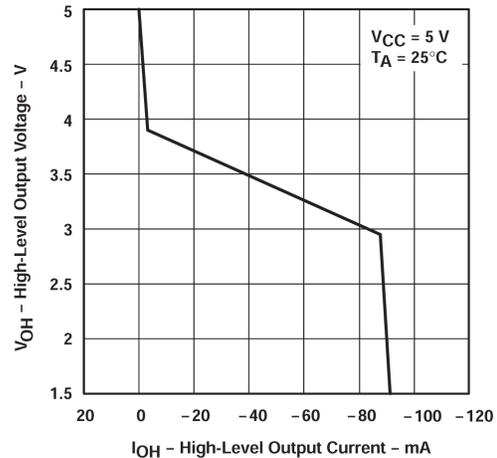
**Figure 5-4. High-level Output Voltage vs High-level Output Current**
