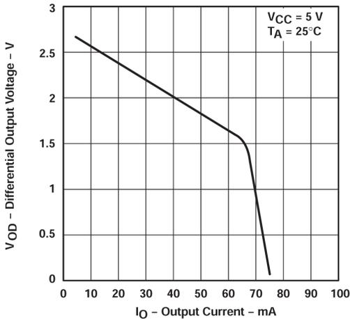
**Figure 5-5. Differential Output Voltage vs Output Current**
