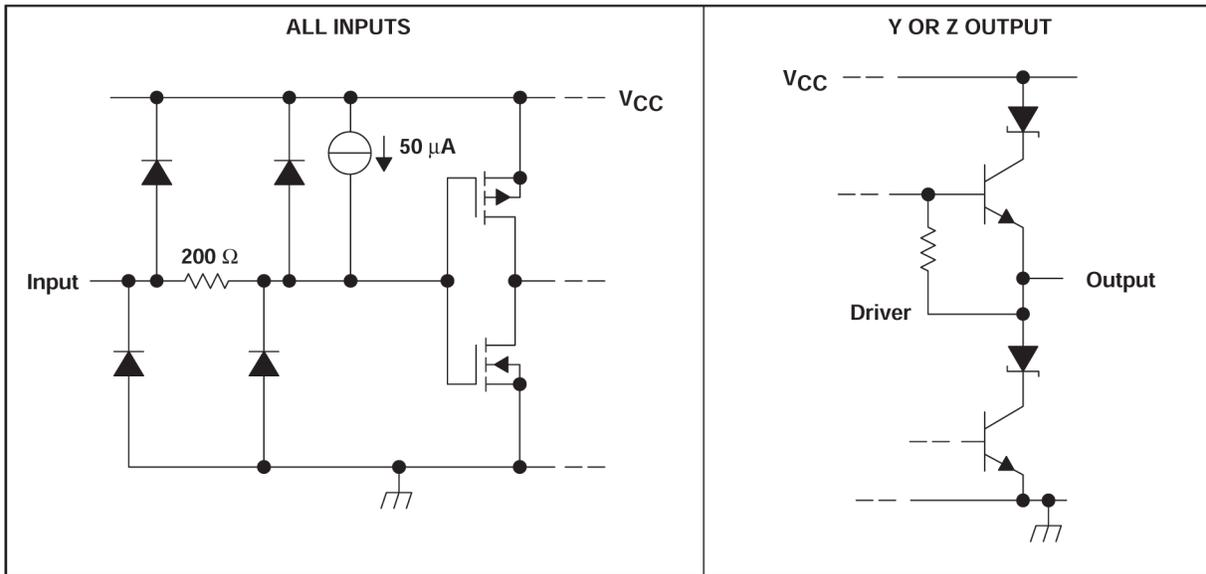
**Figure 7-2. Schematic Diagrams of Inputs and Outputs**
