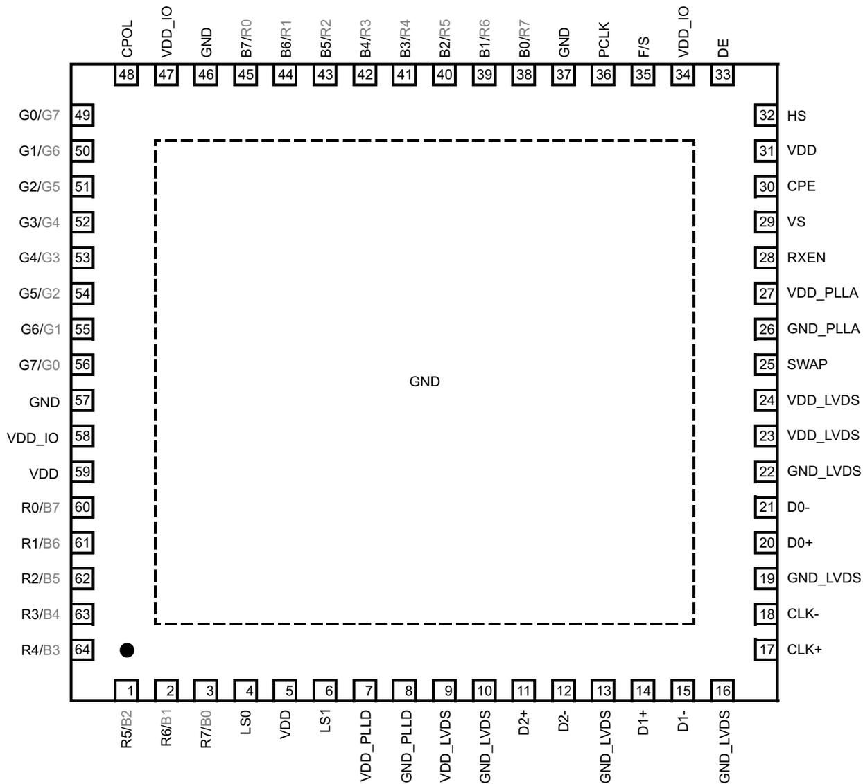
RGB output pin assignment based on SWAP pin setting:
