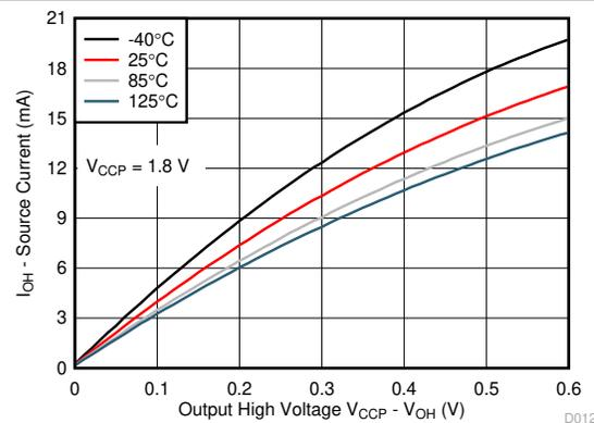
Figure 6-12. I/O Source Current vs Output High Voltage (V<sub>C<sub>CP</sub></sub> = 1.8 V)
