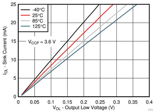
Figure 6-9. I/O Sink Current vs Temperature (V<sub>C<sub>CP</sub></sub> = 3.6 V)
