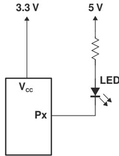
**Figure 9-3. Device Supplied by a Low Voltage**
