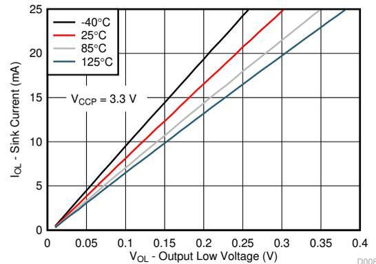
Figure 6-8. I/O Sink Current vs Output Low Voltage (V<sub>C<sub>CP</sub></sub> = 3.3 V)
