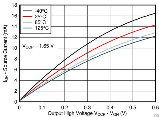
Figure 6-11. I/O Source Current vs Output High Voltage (V<sub>C<sub>CP</sub></sub> = 1.65 V)
