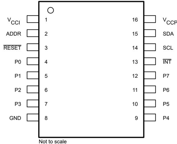
**Figure 5-1. PW Package, 16-Pin TSSOP
