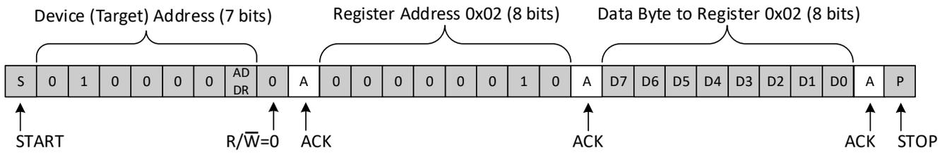
Figure 8-6. Write to the Polarity Inversion Register
