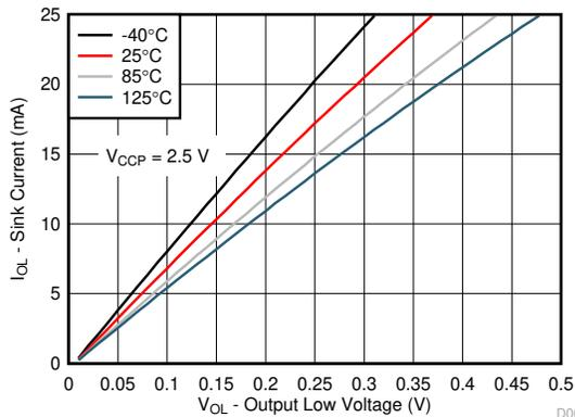
Figure 6-7. I/O Sink Current vs Output Low Voltage (V<sub>C<sub>CP</sub></sub> = 2.5 V)
