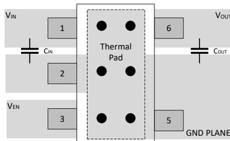
**Figure 7-9. Layout Example: DYD Package**
