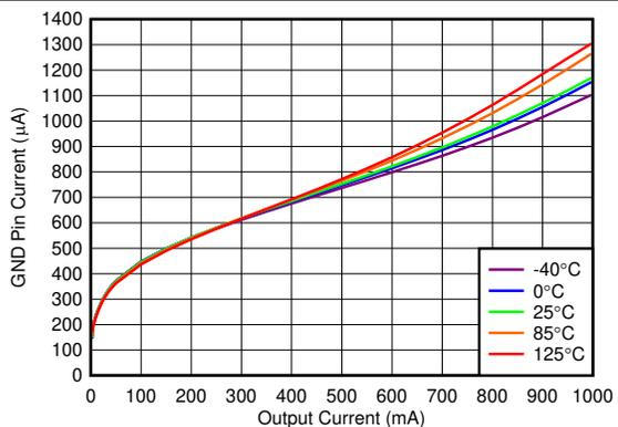
Figure 5-18.  $I_{GND}$  vs  $I_{OUT}$
