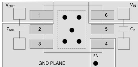
**Figure 7-8. Layout Example: DRV Package**
