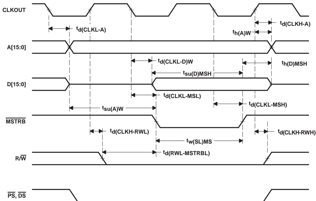
Figure 17. Memory Write ( $\overline{\text{MSTRB}} = 0$ )
