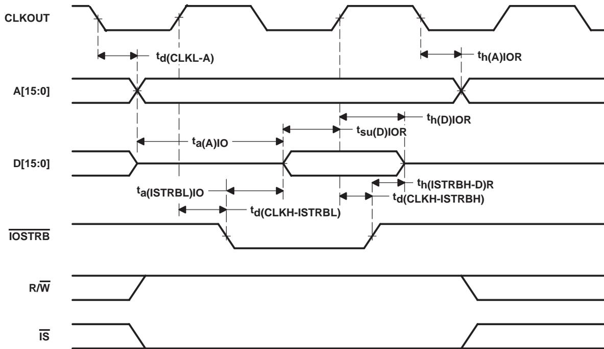
Figure 18. Parallel I/O Port Read ( $\overline{\text{IOSTRB}} = 0$ )
