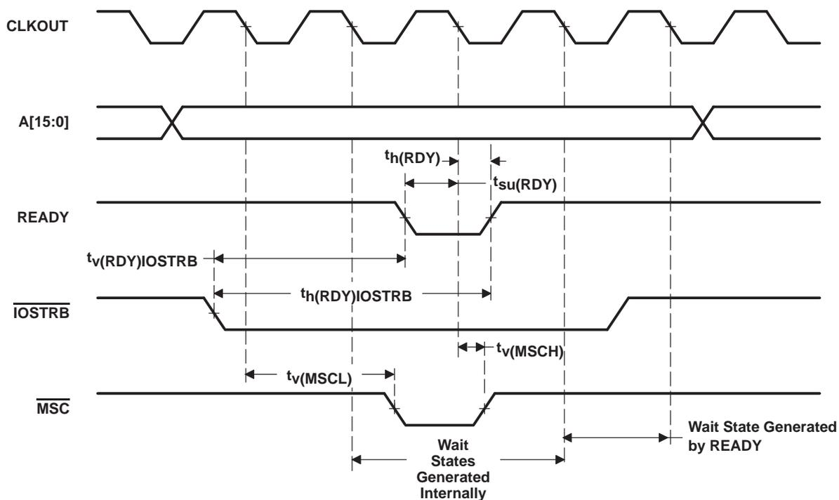
Figure 23. I/O Read With Externally Generated Wait States
