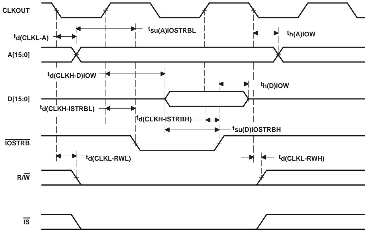
Figure 19. Parallel I/O Port Write ( $\overline{IOSTRB} = 0$ )
