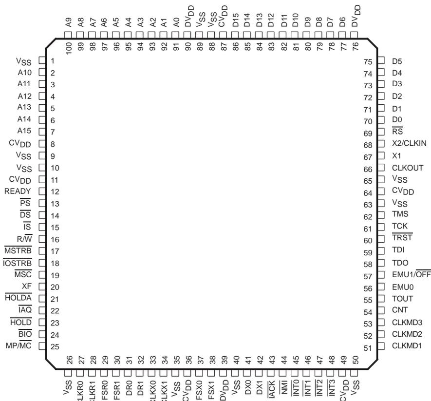
† DV<sub>DD</sub> is the power supply for the I/O pins while CV<sub>DD</sub> is the power supply for the core CPU, and V<sub>SS</sub> is the ground for both the I/O pins and the core CPU.
