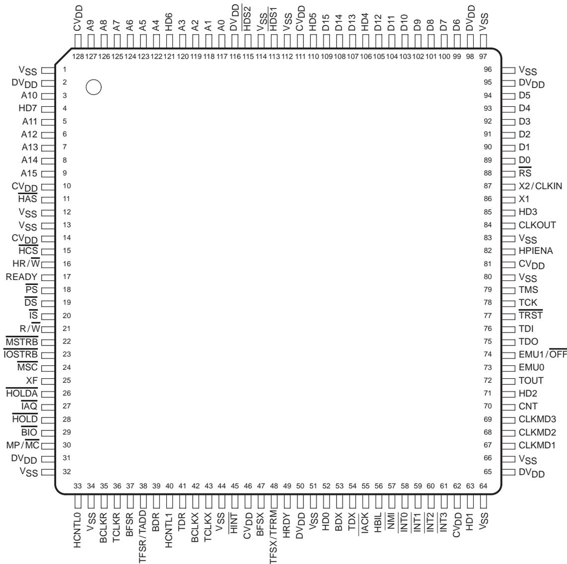
† DVDD is the power supply for the I/O pins while CVDD is the power supply for the core CPU, and VSS is the ground for both the I/O pins and the core CPU.
