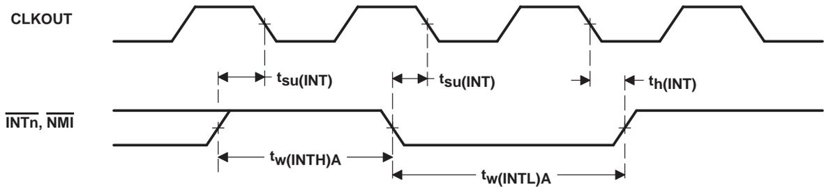
Figure 27. Interrupt Timing
