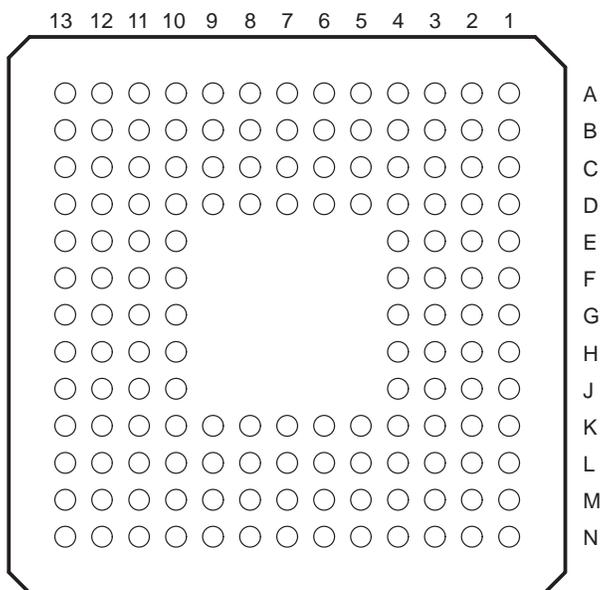
The pin assignments table to follow lists each signal quadrant and BGA ball pin number for the TMS320LC548, TMS320LC549, and TMS320VC549 (144-pin BGA package).
