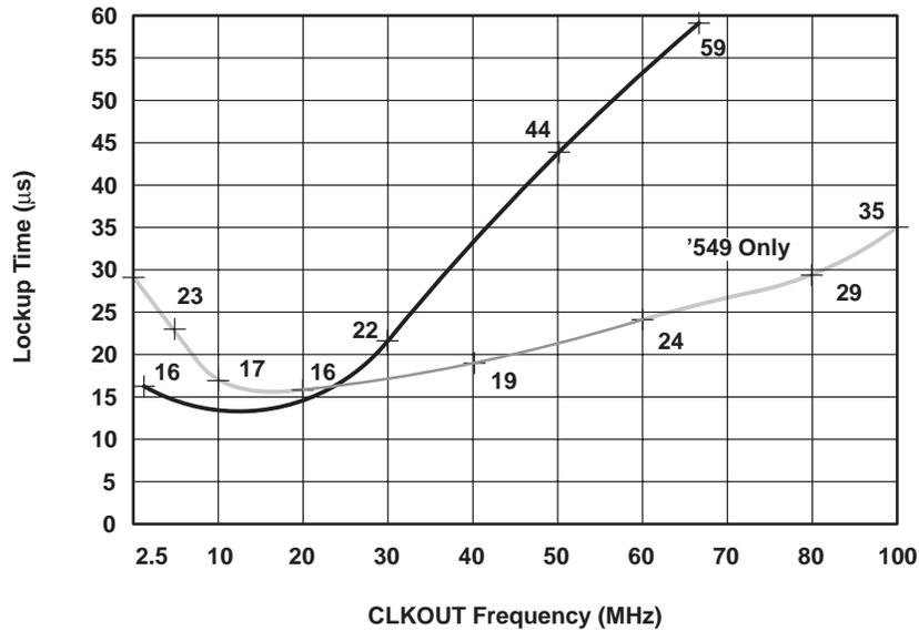
**Figure 8. PLL Lockup Time Versus CLKOUT Frequency**
