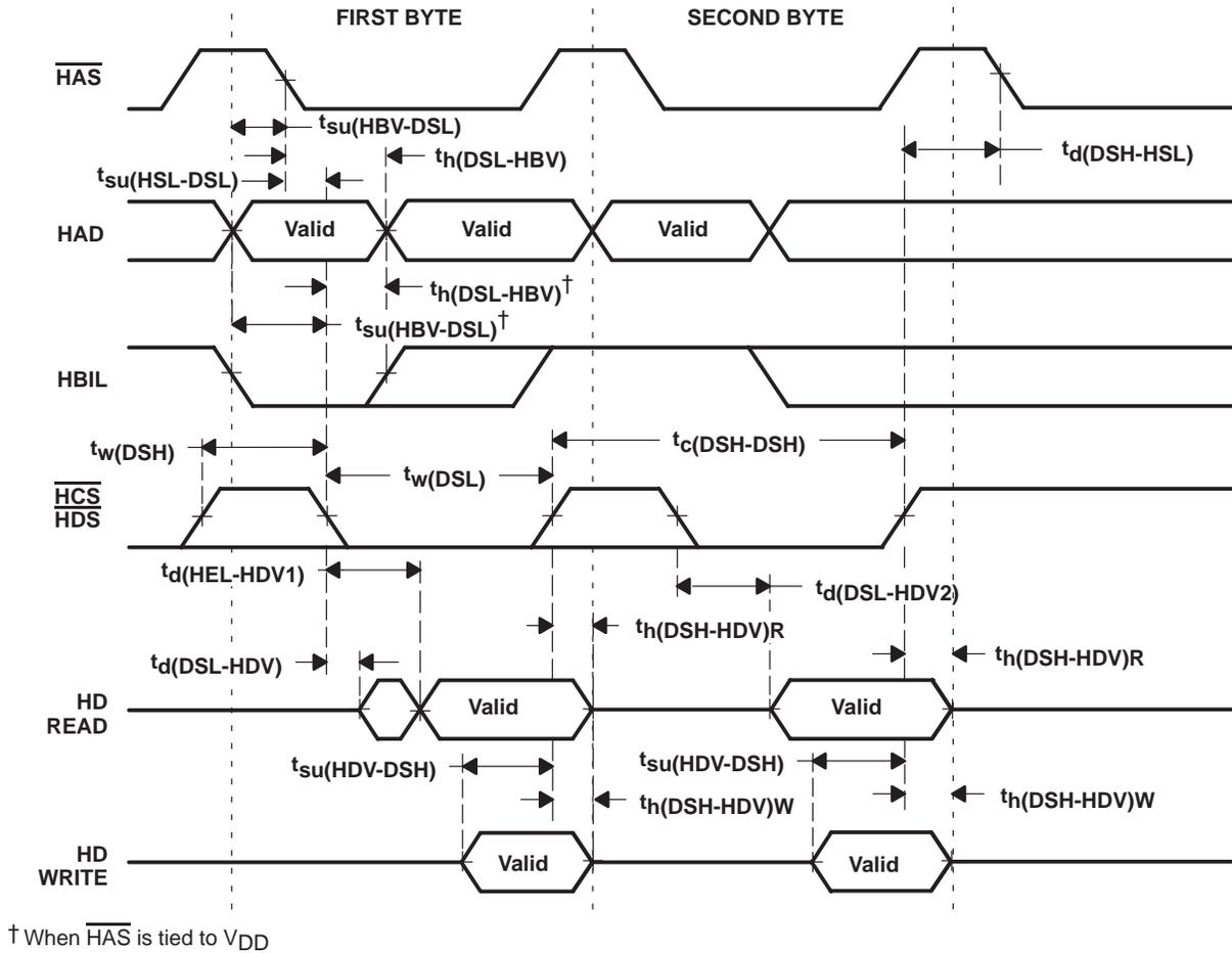
Figure 41. Read/Write Access Timings Using  $\overline{\text{HAS}}$  Without HRDY
