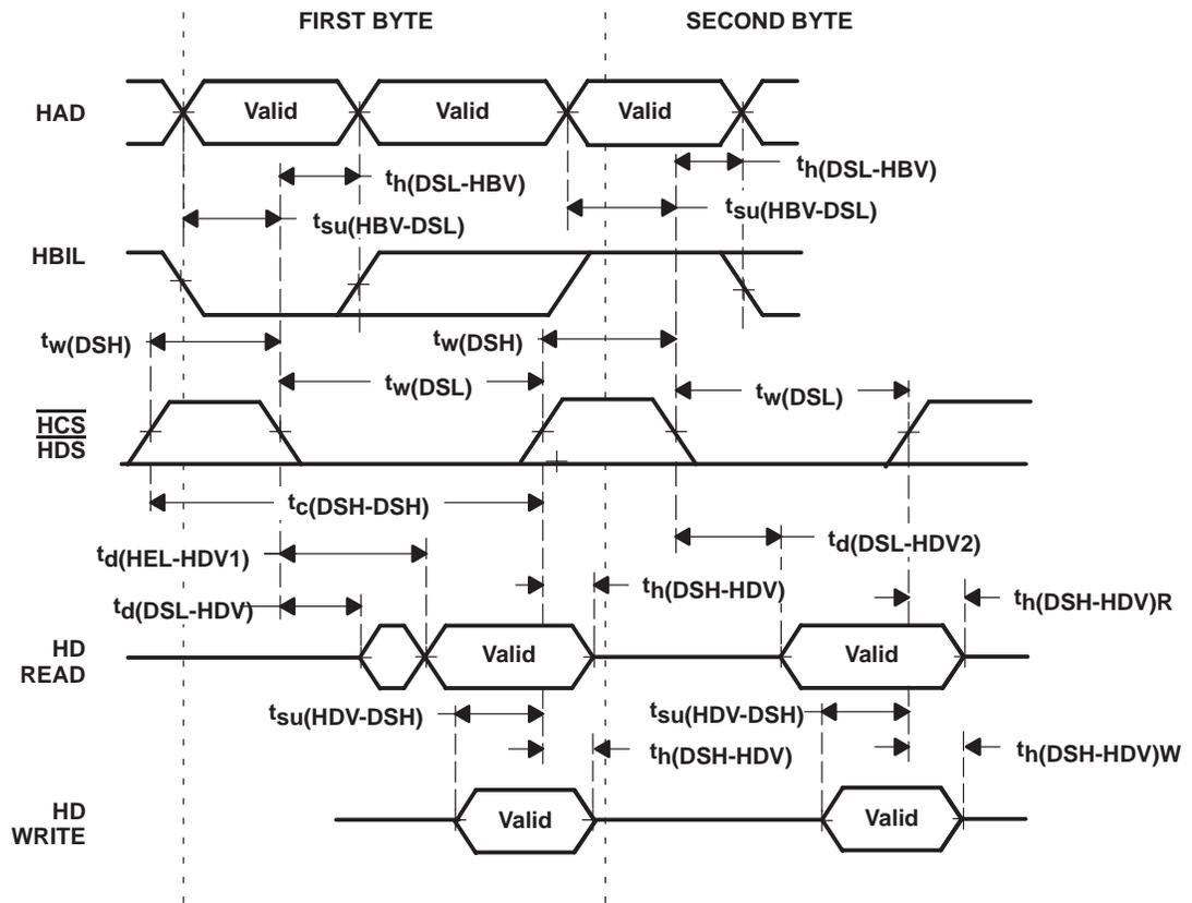
Figure 40. Read/Write Access Timings Without HRDY or  $\overline{\text{HAS}}$
