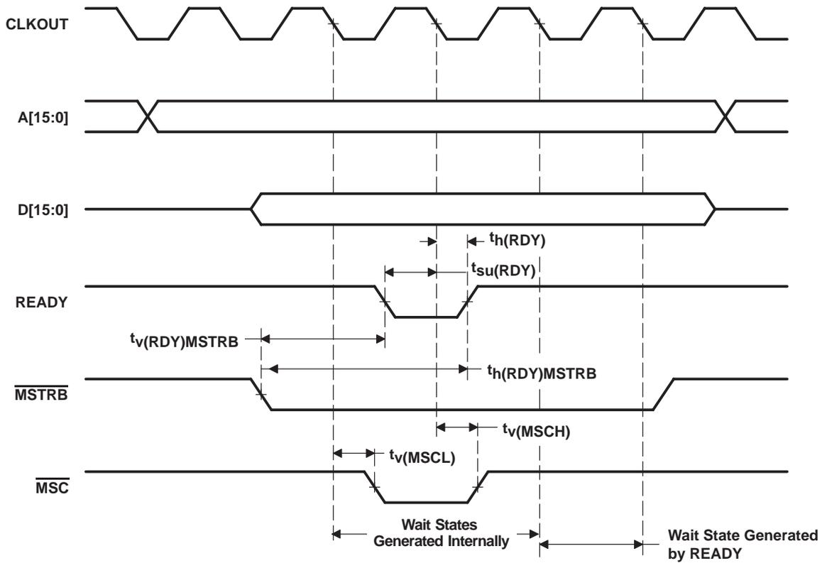
Figure 22. Memory Write With Externally Generated Wait States
