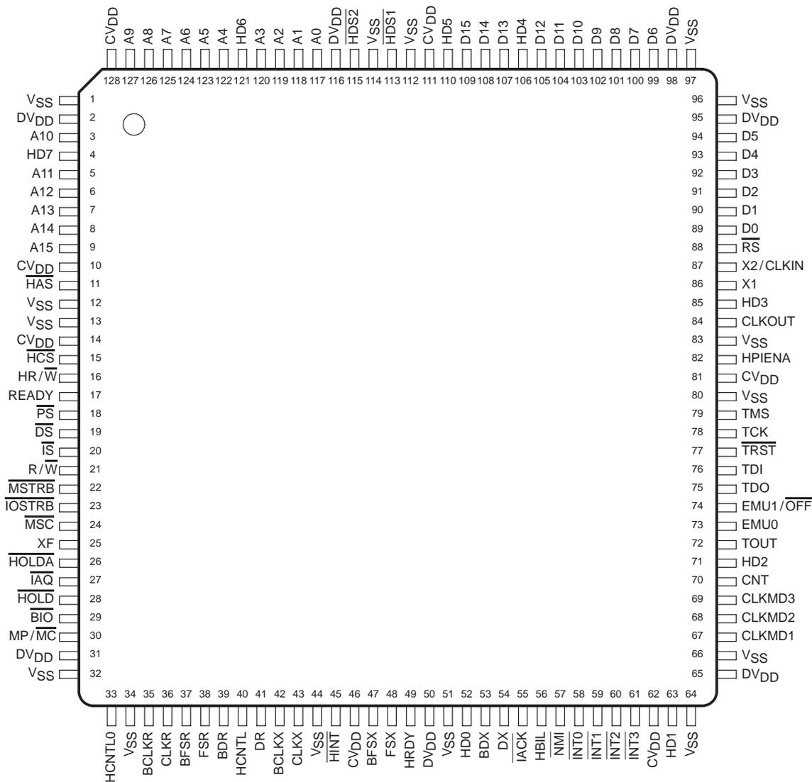
†  $DV_{DD}$  is the power supply for the I/O pins while  $CV_{DD}$  is the power supply for the core CPU, and  $V_{SS}$  is the ground for both the I/O pins and the core CPU.
