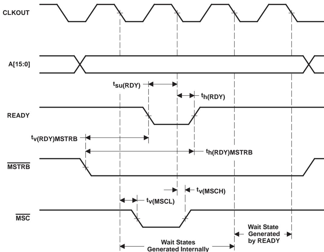
Figure 21. Memory Read With Externally Generated Wait States
