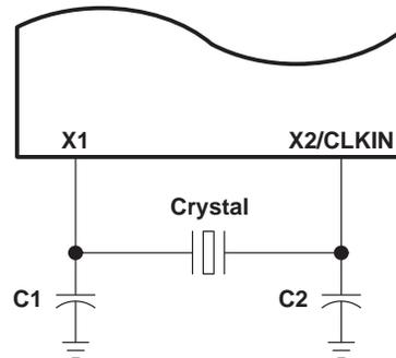
Figure 13. Internal Divide-by-Two Clock Option With External Crystal
