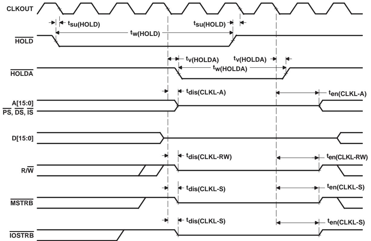
Figure 25.  $\overline{HOLD}$  and  $\overline{HOLDA}$  Timing (HM = 1)
