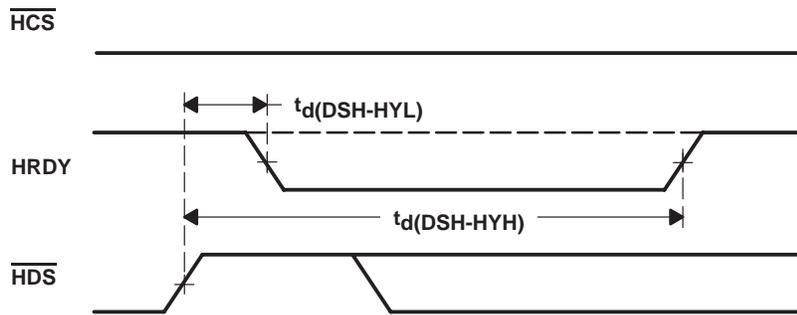
Figure 43. HRDY Signal When  $\overline{\text{HCS}}$  is Always Low
