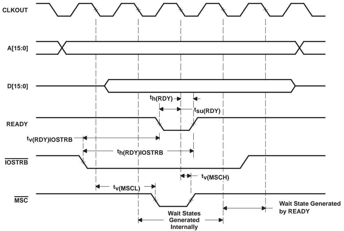
Figure 24. I/O Write With Externally Generated Wait States
