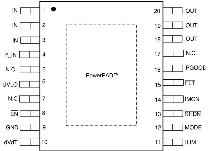
Figure 5-2. TPS16530 PWP Package 20-Pin HTSSOP Top View
