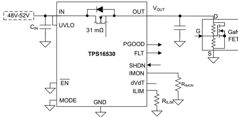
**Figure 9-8. TPS16530 Configured for 48-V Power Amplifier Protection**
