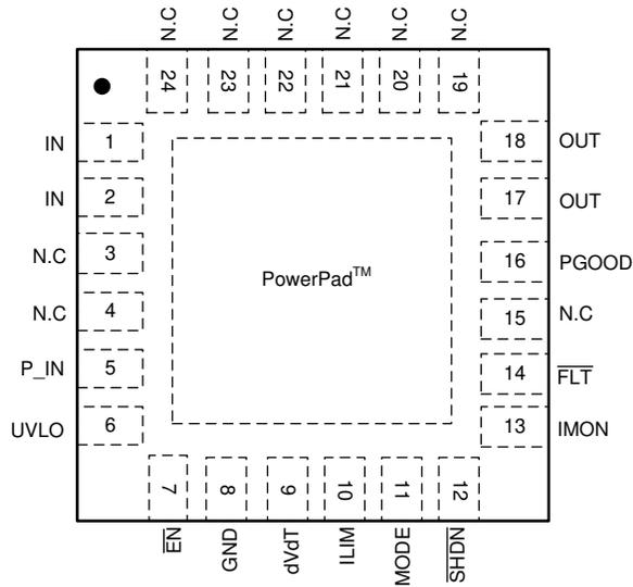
Figure 5-1. TPS16530 RGE Package 24-Pin VQFN Top View
