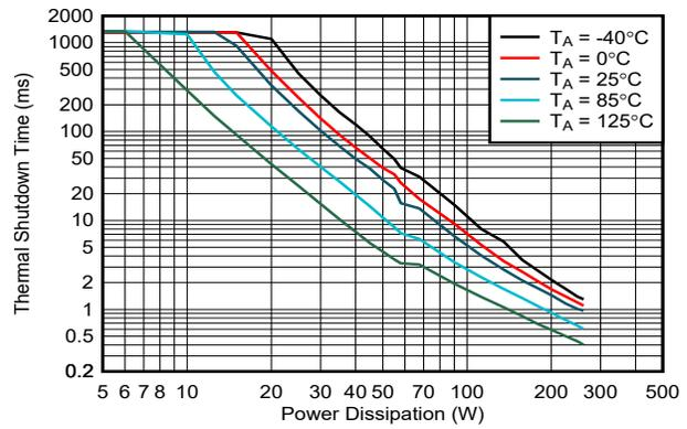
Taken on HTSSOP with 110 cm<sup>2</sup> copper connected to Exposed PAD
