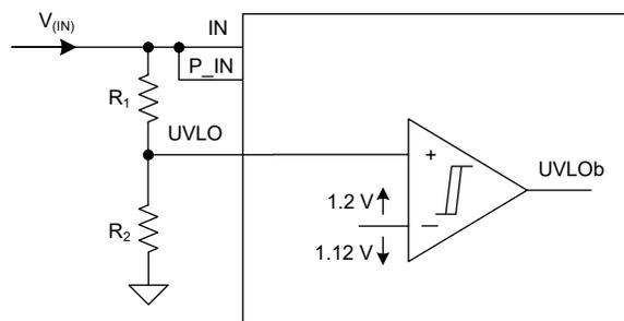
Figure 8-3. UVLO Thresholds Set by  $R_1$  and  $R_2$
