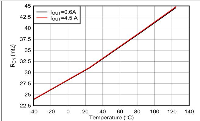
Figure 6-1. On-Resistance vs Temperature Across Load Current
