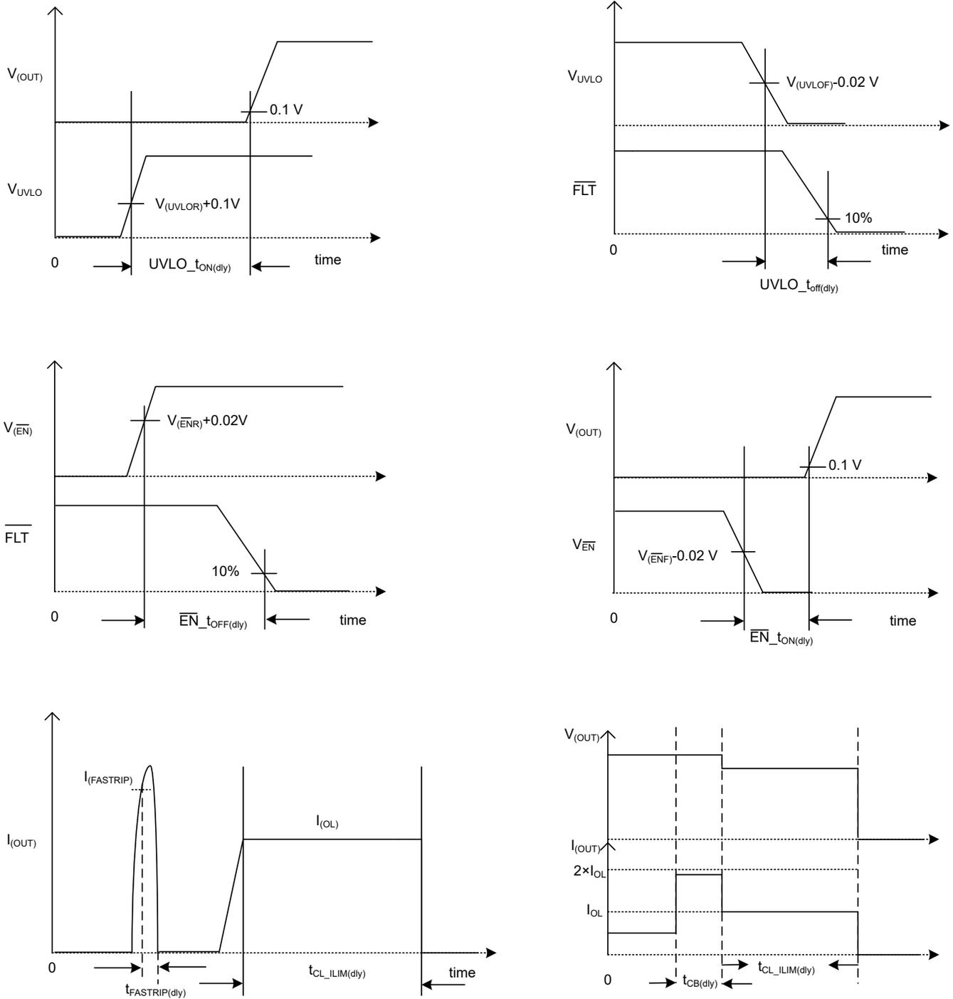
**Figure 7-1. Timing Waveforms**
