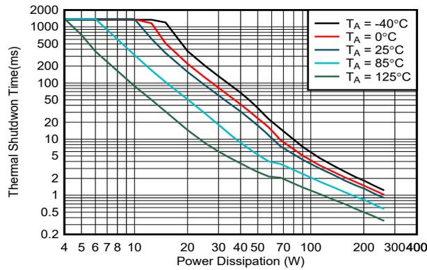
Taken on VQFN device with 95 cm<sup>2</sup> copper connected to Exposed PAD
