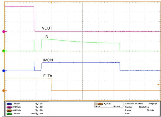
**Figure 9-5. Output Hot-short Performance with 50-V Input Supply**
