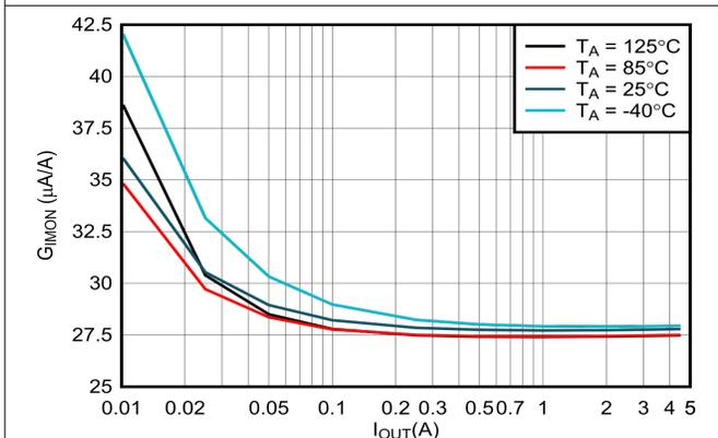
Figure 6-5. Current Monitor Gain vs Output Current
