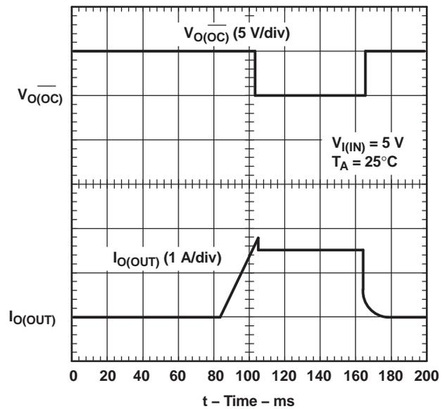
Figure 7. TPS2032, Ramped Load on Enabled Device
