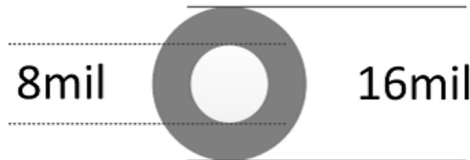
Figure 11-6. Recommended Minimum Via Sizing
