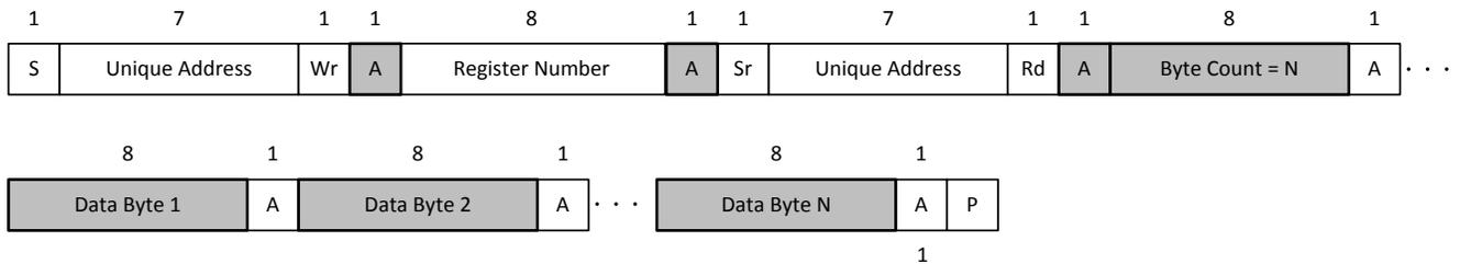
**Figure 8-11. I<sup>2</sup>C Unique Address Read Register Protocol**
