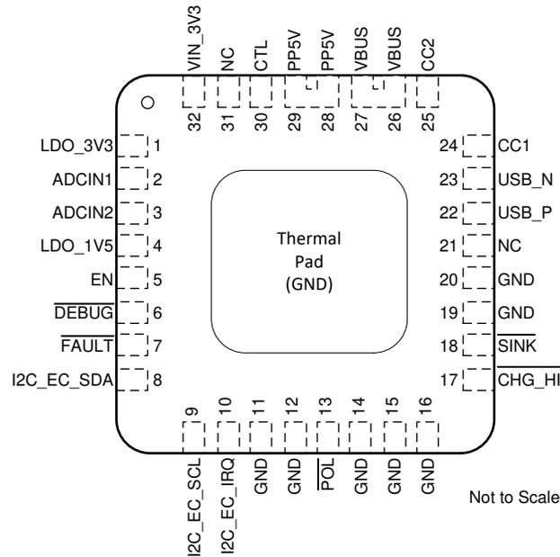
**Figure 5-1. RSM Package 32-pin QFN Top View**
