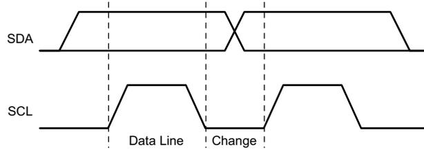
Figure 8-8. I<sup>2</sup>C Bit Transfer
