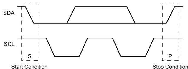
**Figure 8-7. I<sup>2</sup>C Definition of Start and Stop Conditions**
