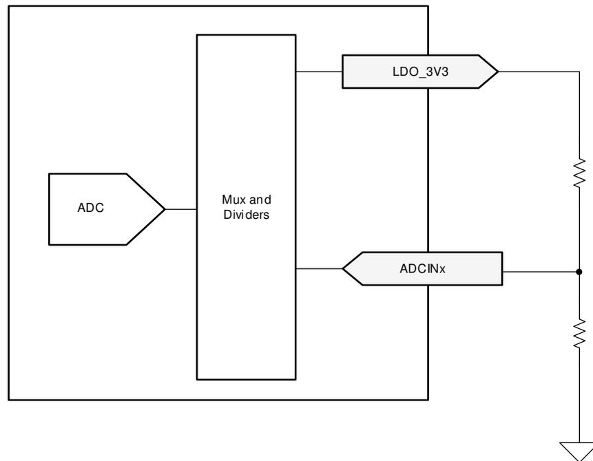
Figure 8-4. ADCINx Resistor Divider
