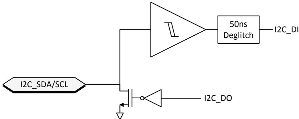
**Figure 8-6. I<sup>2</sup>C Buffer**
