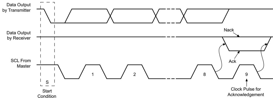
Figure 8-9. I<sup>2</sup>C Acknowledgment
