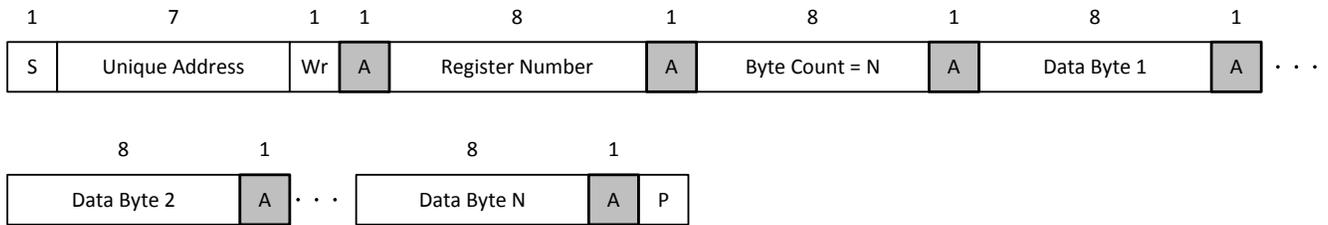
**Figure 8-10. I<sup>2</sup>C Unique Address Write Register Protocol**
