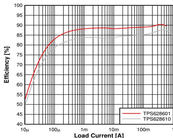
Efficiency Versus I<sub>OUT</sub> at 1.1 V<sub>OUT</sub>, 3.8 V<sub>IN</sub>
