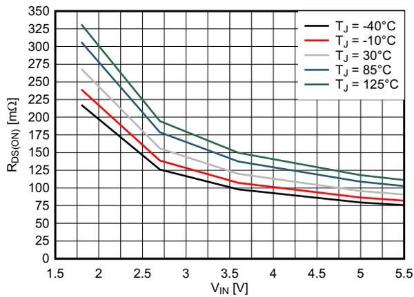
Figure 7-3. High-side Switch Drain Source Resistance  $R_{DS(ON)}$
