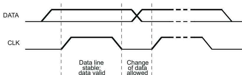
Figure 8-4. Bit Transfer on the Serial Interface
