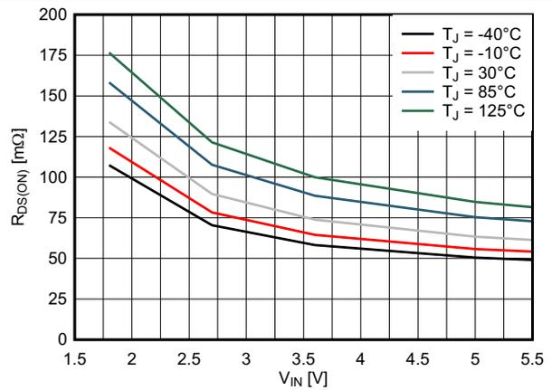
Figure 7-4. Low-side Switch Drain Source Resistance  $R_{DS(ON)}$
