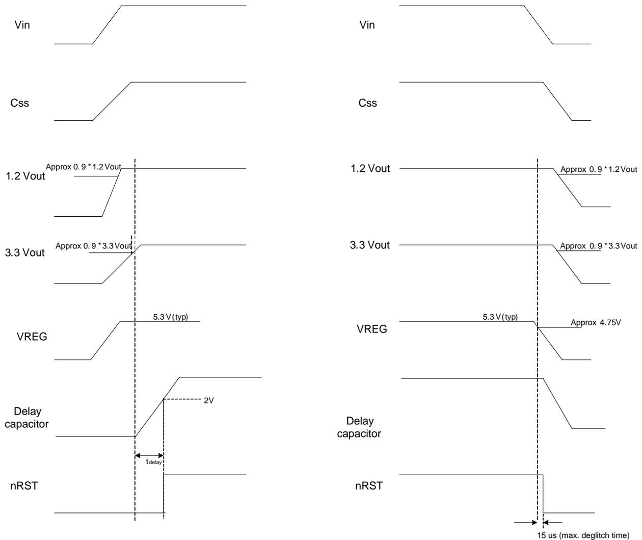
On power up, ALL three regulated supplies, VREG, 3.3 V, and 1.234 V, must be more than 90% of their respective values before the delay timer capacitor on the DELAY pin can start charging.
