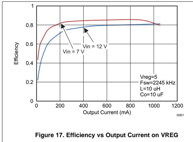
Figure 17. Efficiency vs Output Current on VREG
