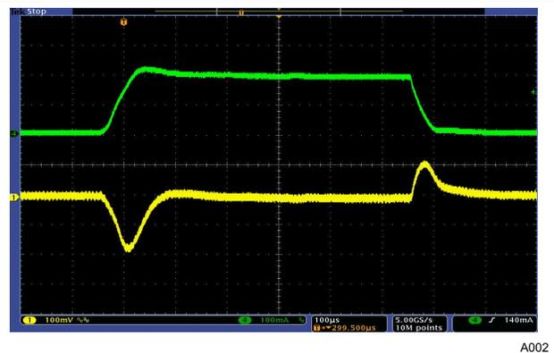
Figure 18. Load Transient Response, 10 mA to 200 mA
