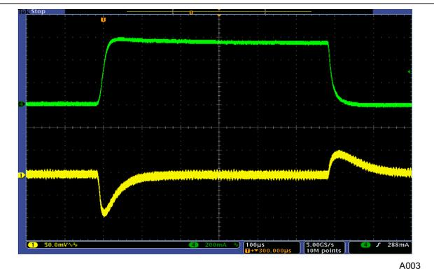
Figure 20. Load Transient Response, 10 mA to 550 mA
