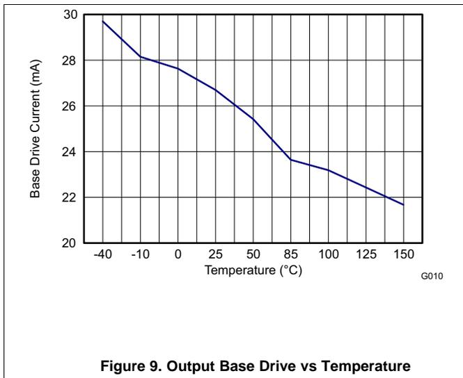
Figure 9. Output Base Drive vs Temperature
