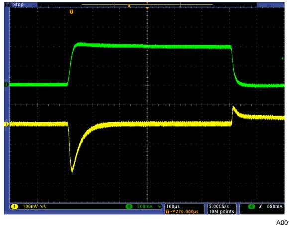
Figure 21. Load Transient Response, 10 mA to 1 A
