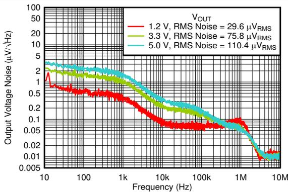
$V_{IN} = V_{OUT(nom)} + 1\text{ V}$ ,  $I_{OUT} = 300\text{ mA}$ ,  $V_{RMS}\text{ BW} = 10\text{ Hz to }100\text{ kHz}$
