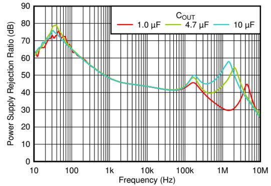
$V_{IN} = 6\text{ V}$ ,  $C_{IN} = 0\ \mu\text{F}$ ,  $V_{OUT} = 5.0\text{ V}$ ,  $I_{OUT} = 300\text{ mA}$
