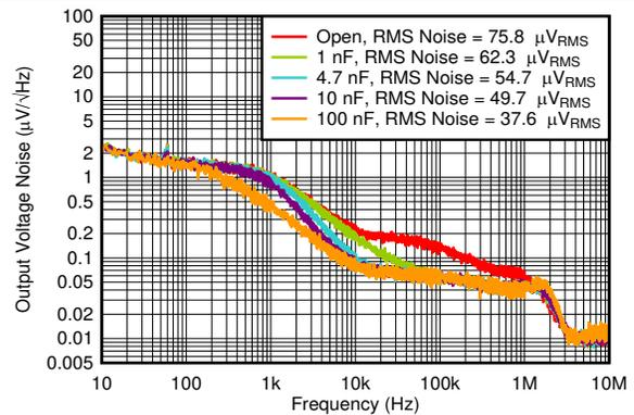
$V_{IN} = 4.3\text{ V}$ ,  $V_{OUT} = 3.3\text{ V}$ ,  $I_{OUT} = 300\text{ mA}$ ,  $V_{RMS}\text{ BW} = 10\text{ Hz to }100\text{ kHz}$
