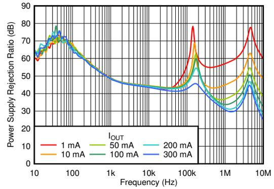
$V_{IN} = 6\text{ V}$ ,  $C_{IN} = 0\ \mu\text{F}$ ,  $V_{OUT} = 5.0\text{ V}$
