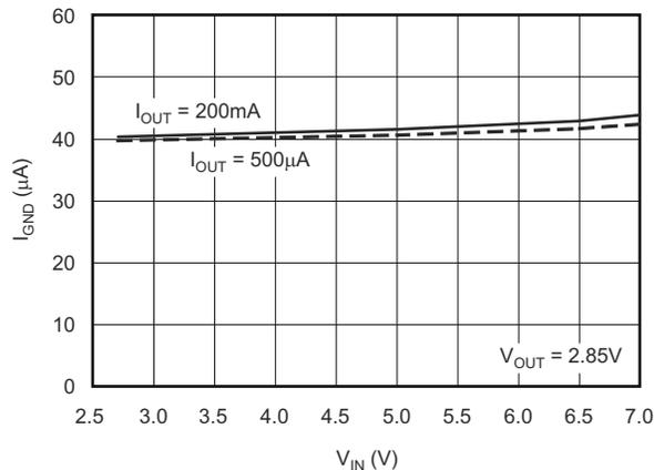
Figure 6-5. Ground Pin Current vs Input Voltage
