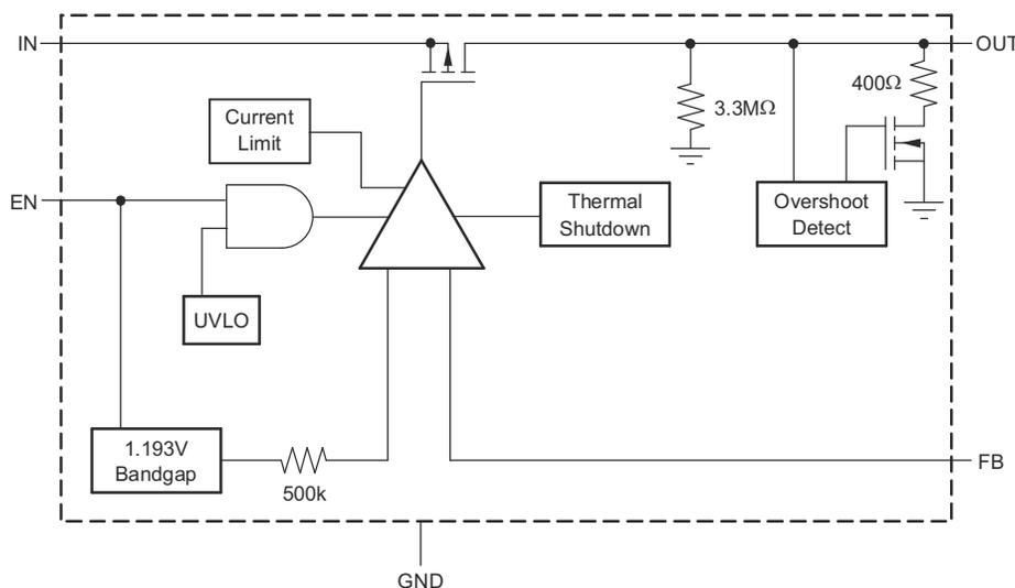
Figure 7-2. Adjustable-Voltage Version
