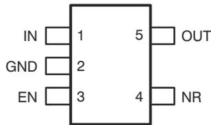
**Figure 5-1. DDC Package, 5-Pin SOT-23 (Top View)**
