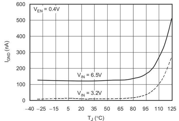
Figure 6-6. Ground Pin Current (Disabled) vs Junction Temperature
