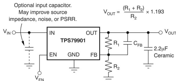
Figure 8-2. Typical Application Circuit for Adjustable-Voltage Version
