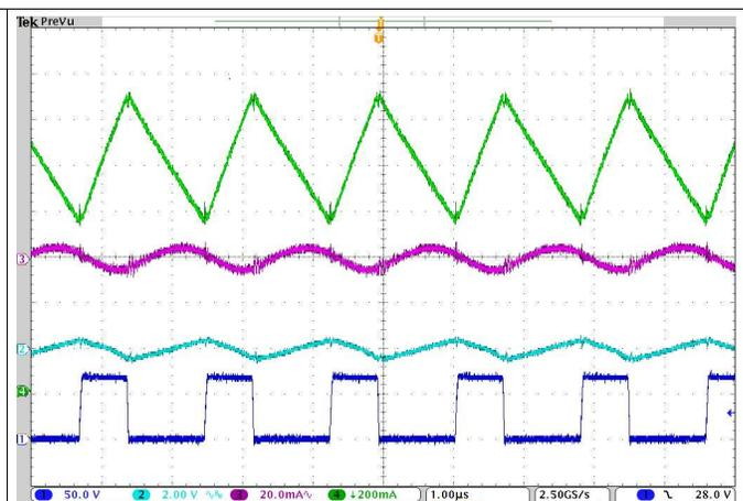
Ch1: SW Voltage; Ch2: VIN Ripple Voltage (AC Coupled);
