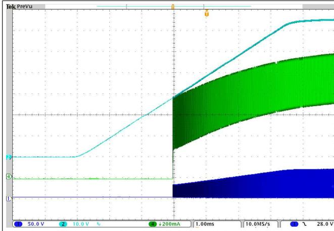
Ch1: SW Voltage; Ch2: VIN (DC Coupled);
