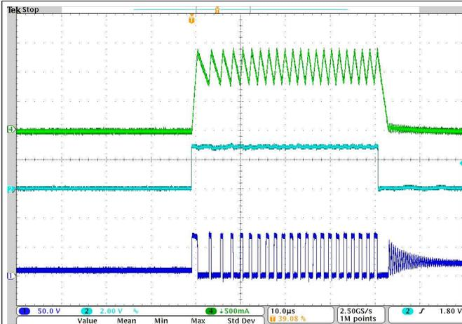
Ch1: SW Voltage; Ch2: PWM pin;
