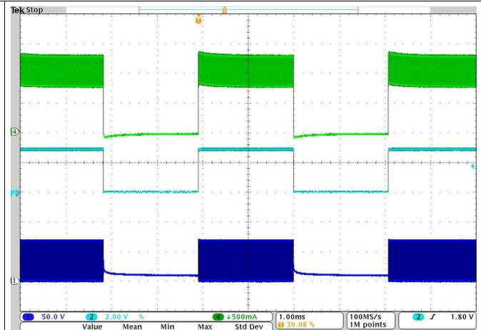
Ch1: SW Voltage; Ch2: PWM pin;
