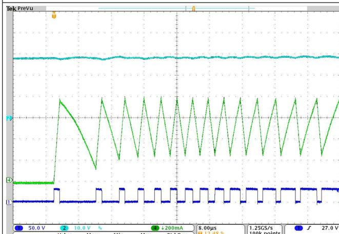
Ch1: SW Voltage; Ch2: VIN (DC Coupled);
