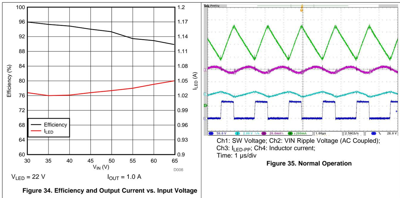
Figure 34. Efficiency and Output Current vs. Input Voltage
