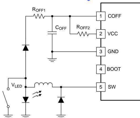
Figure 14. Shunt Dimming COFF Connection
