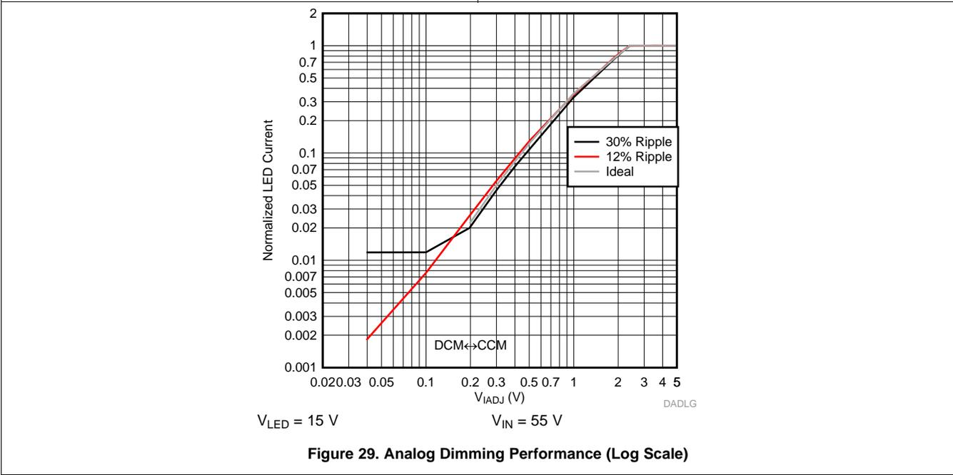
Figure 29. Analog Dimming Performance (Log Scale)
