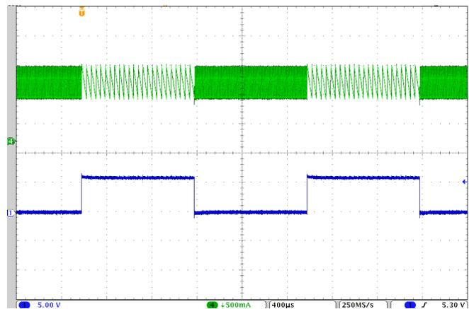
Ch1: PWM Signal Time: 400 μs/div
