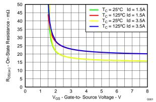
Figure 7. On Resistance vs. Gate Voltage
