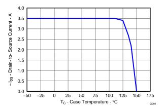
Figure 11. Maximum Drain Current vs. Temperature
