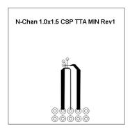
Max  $R_{\theta JA} = 295.5^{\circ} C/W$  when mounted on minimum pad area of 2 oz. Cu.
