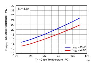
Figure 12. On Resistance vs. Temperature
