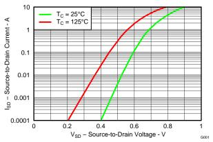
Figure 9. Typical Diode Forward Voltage
