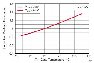
Figure 8. Normalized On Resistance vs. Temperature
