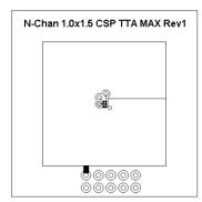
Max  $R_{\theta JA} = 94.6^{\circ}$ C/W when mounted on 1 inch<sup>2</sup> of 2 oz. Cu.
