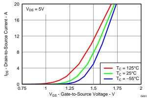
Figure 3. Transfer Characteristics
