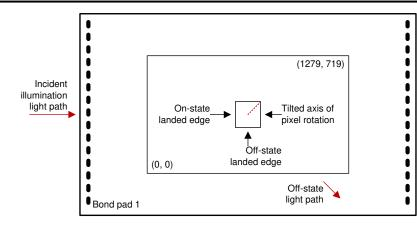
Figure 6-18. Landed Pixel Orientation and Tilt
