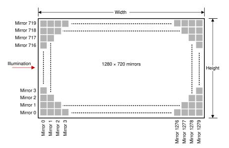
Figure 6-16. Micromirror Array Physical Characteristics
