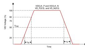
Figure 6-5. SubLVDS Input Rise and Fall Slew Rate
