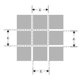
Figure 6-17. Mirror (Pixel) Pitch
