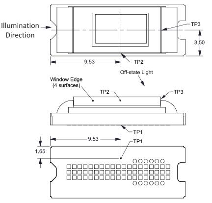
Figure 7-1. Thermal Test Point Location - FQK Package
