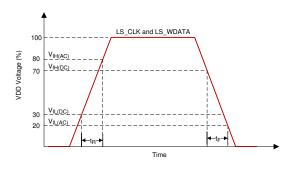
Figure 6-3. LPSDR Input Slew Rate
