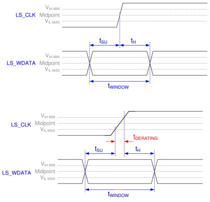
Figure 6-6. Window Time Derating Concept
