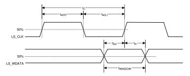
Low-speed interface is LPSDR and adheres to the Section 6.6 and AC/DC Operating Conditions table in JEDEC Standard No. 209B, Low Power Double Data Rate (LPDDR) JESD209B.
