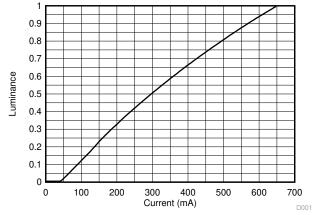
Figure 8-3. Optical Output vs LED Current
