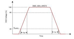
Figure 6-4. LPSDR Input Slew Rate
