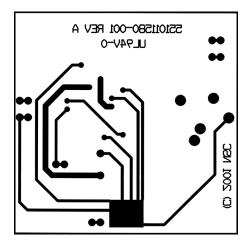
Figure 30. Recommended SOIC PC Board Layout:
