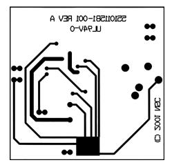
Figure 33. Recommended VSSOP PC Board Layout:
