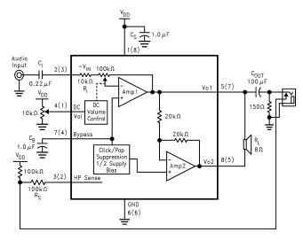
Figure 1. Typical Audio Amplifier Application Circuit
