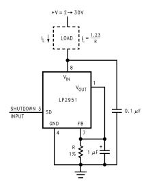
Figure 39. Low Drift Current Source
