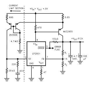
$$V_{out} = 1.23V \left( 1 + \frac{R_1}{R_2} \right)$$
