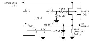
Figure 37. 300mA Regulator with 0.75V Dropout
