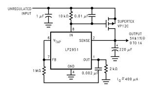
Figure 36. 1A Regulator with 1.2V Dropout
