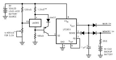
For values shown, Regulator shuts down when  $V_{in}$  < 5.5V and turns on again at 6.0V. Current drain in disconnected mode is  $\approx$  150 $\mu$ A.
