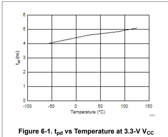
Figure 6-1.  $t_{pd}$  vs Temperature at 3.3-V  $V_{CC}$
