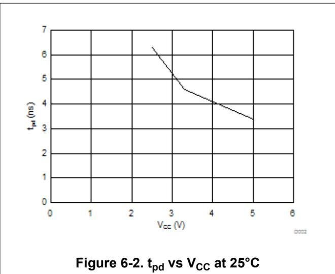
Figure 6-2.  $t_{pd}$  vs  $V_{CC}$  at 25°C
