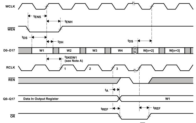
NOTES: A. tSKEW1 is the minimum time between a rising WCLK edge and a rising RCLK edge for  $\overline{OR}$  to go high during the current cycle. If the time between the rising edge of WLCK and the rising edge of RCLK is less than tSKEW1, the  $\overline{OR}$  deassertion might be delayed one extra RCLK cycle.
