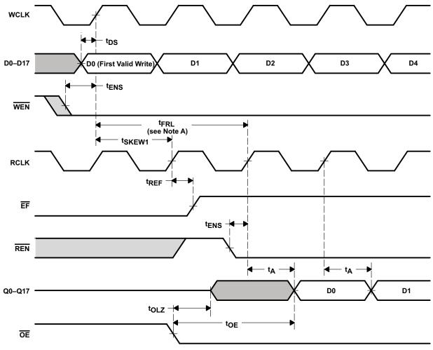
NOTES: A. When  $t_{SKEW1}$  is at the minimum specification,  $t_{FRL}$  (maximum) =  $t_{CLK}$  +  $t_{SKEW1}$ . When  $t_{SKEW1}$  is less than the minimum specification, t<sub>FRL</sub> (maximum) = either (2 ×t<sub>CLK</sub>) + t<sub>SKEW1</sub> or t<sub>CLK</sub> + t<sub>SKEW1</sub>. The latency timing applies only at the empty boundary (EF is low).
