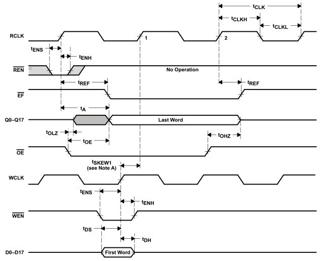
NOTES: A. t<sub>SKEW1</sub> is the minimum time between a rising WCLK edge and a rising RCLK edge to ensure that  $\overline{\text{EF}}$  goes high after one RCLK cycle plus t<sub>REF</sub>. If the time between the rising edge of WCLK and the rising edge of RCLK is less than t<sub>SKEW1</sub>, the  $\overline{\text{EF}}$  deassertion might be delayed an extra RCLK cycle.
