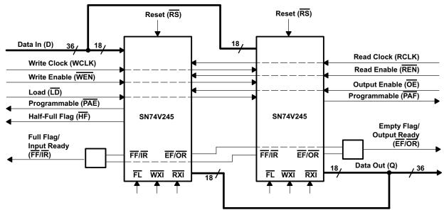
NOTE A: Do not connect any output control signals directly together.
