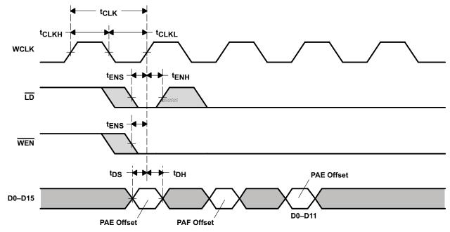
Figure 9. Write Programmable Registers (Standard and FWFT Modes)
