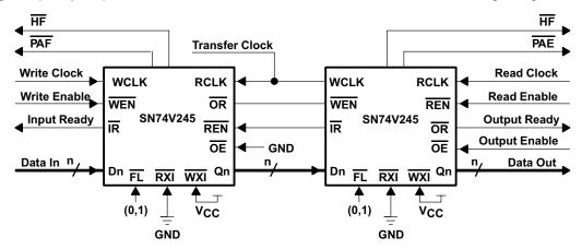
Figure 29. Block Diagram of 8192 × 18 Synchronous FIFO Memory With Programmable Flags Used in Depth-Expansion Configuration
