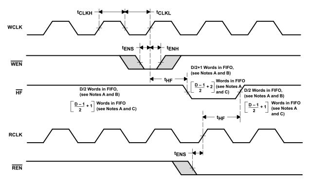
NOTES: A. D = maximum FIFO depth In FWFT mode: D = 4097 In standard mode: D = 4096
