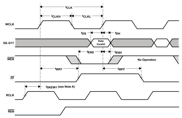
NOTES: A. t<sub>SKEW1</sub> is the minimum time between a rising RCLK edge and a rising WCLK edge to ensure that  $\overline{\text{FF}}$  goes high during the current clock cycle. If the time between the rising edge of RCLK and the rising edge of WCLK is less than t<sub>SKEW1</sub>,  $\overline{\text{FF}}$  might not change state until the next WCLK edge.
