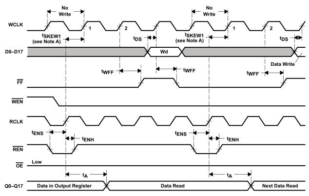
NOTES: A. t<sub>SKEW1</sub> is the minimum time between a rising RCLK edge and a rising WCLK edge to ensure that  $\overline{\text{FF}}$  goes high after one WCLK cycle plus t<sub>WFF</sub>. If the time between the rising edge of RCLK and the rising edge of WCLK is less than t<sub>SKEW1</sub>, the  $\overline{\text{FF}}$  deassertion time might be delayed an extra WCLK cycle.
