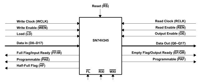
Figure 26. Block Diagram of Single 4096 x 18 Synchronous FIFO
