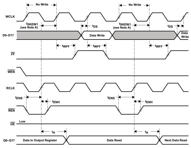
NOTES: A. t<sub>SKEW1</sub> is the minimum time between a rising RCLK edge and a rising WCLK edge to ensure that FF goes high during the current clock cycle. If the time between the rising edge of RCLK and the rising edge of WCLK is less than t<sub>SKEW1</sub>, FF might not change state until the next WCLK edge.
