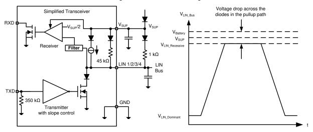
Figure 7-1. Commander Node Configuration with Voltage Levels
