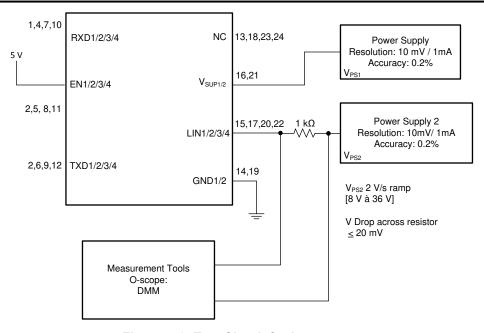
Figure 7-8. Test Circuit for I<sub>BUS\_PAS\_rec</sub>
