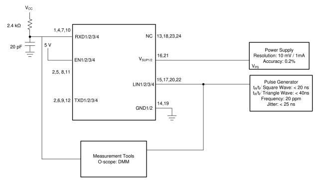
Figure 7-13. Propagation Delay Test Circuit
