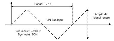
Figure 7-3. LIN Bus Input Signal
