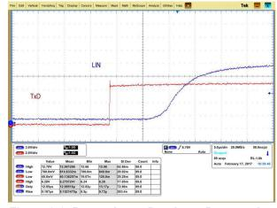
Figure 8-2. Dominant to Recessive Propagation
