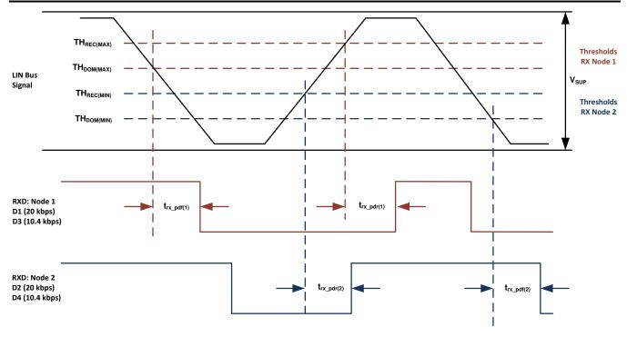
Figure 7-14. Propagation Delay
