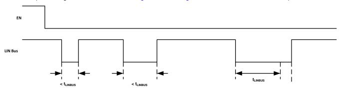
Figure 7-2. No Bus Fault: Entering Sleep Mode with Bus Recessive Condition and Wakeup
