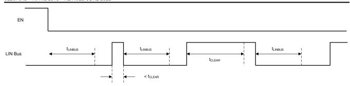
Figure 7-3. Bus Fault: Entering Sleep Mode with Bus Stuck Dominant Fault, Clearing, and Wakeup
