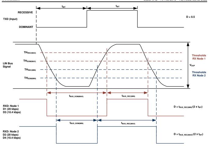
Figure 7-12. Definition of Bus Timing Parameters
