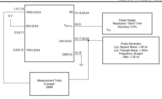
Figure 7-4. LIN Receiver Test with RX Access
