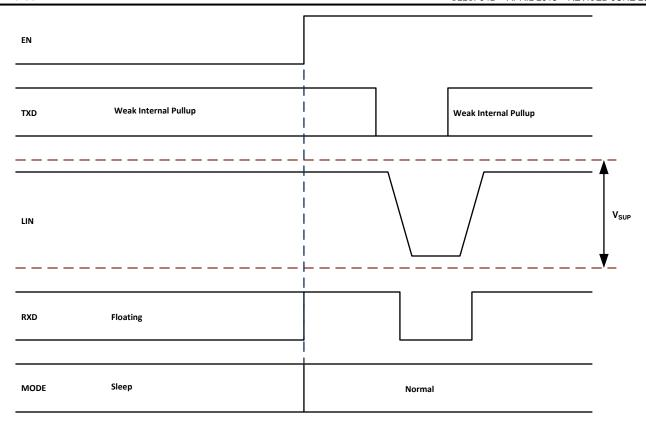
Figure 7-16. Wake Up Through EN
