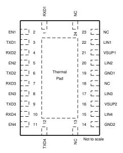
Figure 5-1. RGY Package, 24-Pin RGY (VQFN) (Top View)
