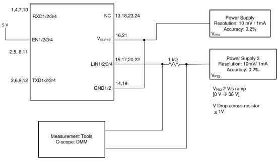
Figure 7-9. Test Circuit for I<sub>BUS NO GND</sub> Loss of GND
