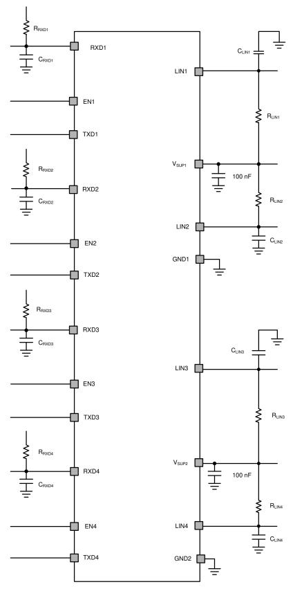
Figure 7-18. Test Circuit for AC Characteristics
