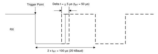
Figure 7-2. RX Response: Operating Voltage Range
