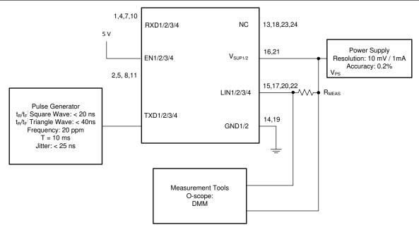
Figure 7-6. Test Circuit for I<sub>BUS\_LIM</sub> at Dominant State (Driver on)
