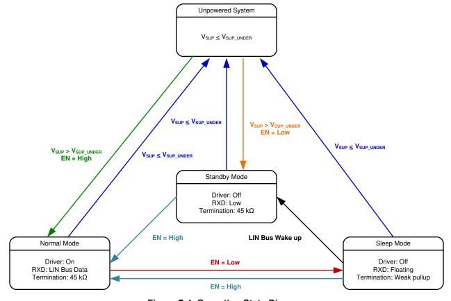
Figure 7-4. Operating State Diagram
