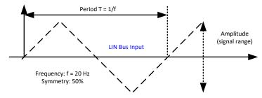
Figure 8-3. LIN Bus Input Signal
