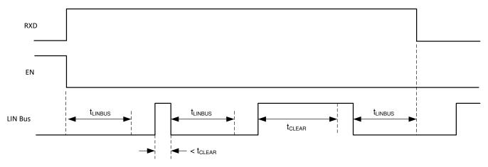
Figure 9-4. Bus Fault: Entering Sleep Mode with Bus Stuck Dominant Fault, Clearing, and Wakeup
