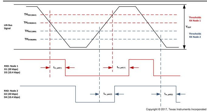
Figure 8-14. Propagation Delay
