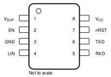
Figure 6-1. D Package, 8-Pin (SOIC), Top View
