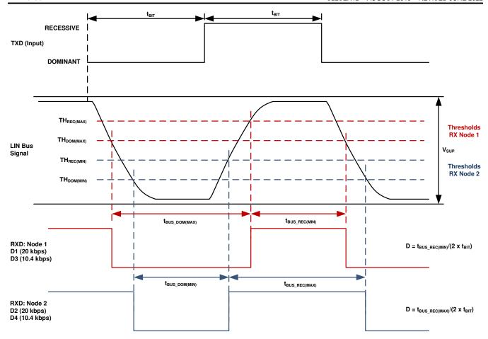
Figure 8-12. Definition of Bus Timing
