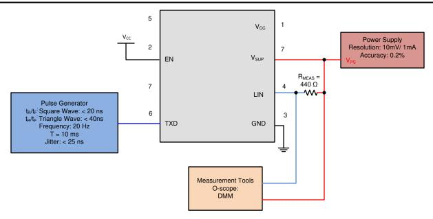
Figure 8-6. Test Circuit for I<sub>BUS\_LIM</sub> at Dominant State (Driver on)
