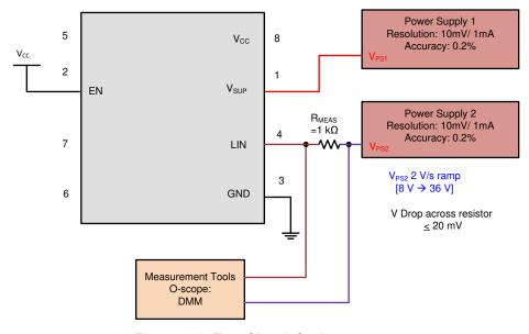
Figure 8-8. Test Circuit for I<sub>BUS\_PAS\_rec</sub>
