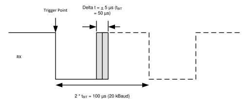
Figure 8-2. RX Response: Operating Voltage Range
