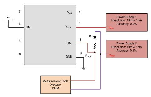
Figure 8-5. V<sub>SUP\_NON\_OP</sub> Test Circuit
