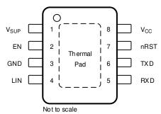
Figure 6-3. DDA Package, 8-Pin (HSOIC), Top View
