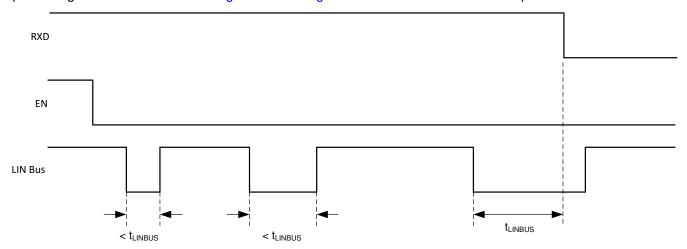
Figure 9-3. No Bus Fault: Entering Sleep Mode with Bus Recessive Condition and Wakeup
