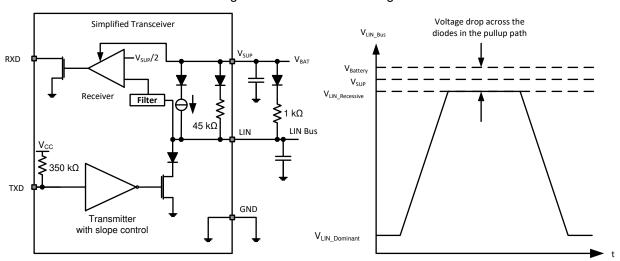
Figure 9-2. Commander Node Configuration with Voltage Levels
