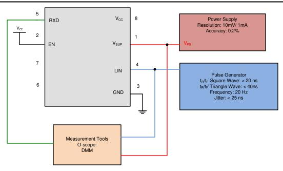
Figure 8-4. LIN Receiver Test with RX access
