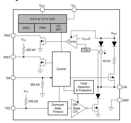
Figure 9-1. Functional Block Diagram
