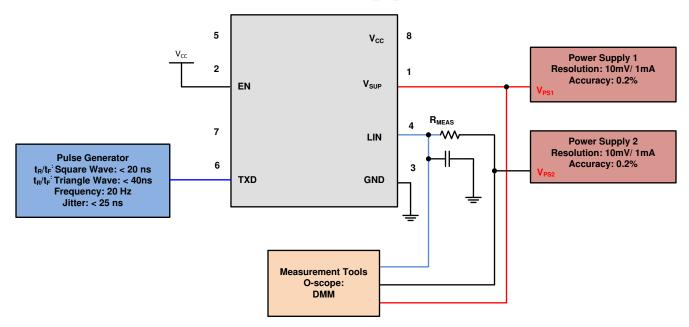
Figure 8-11. Test Circuit Slope Control and Duty Cycle
