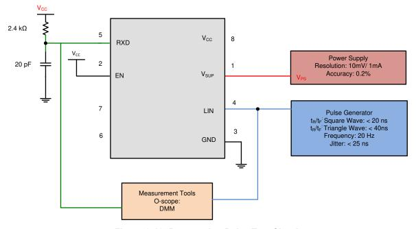
Figure 8-13. Propagation Delay Test Circuit
