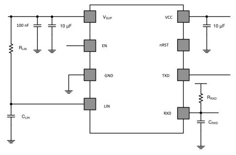
Figure 8-18. Test Circuit for AC Characteristics
