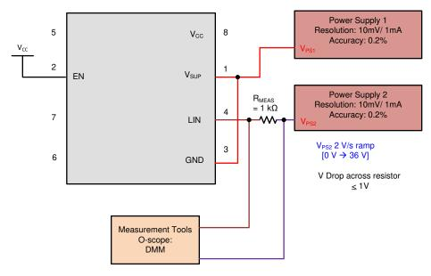
Figure 8-9. Test Circuit for I<sub>BUS\_NO\_GND</sub> Loss of GND
