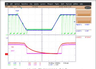
Figure 10-16. Recessive to Dominant Propagation Delay
