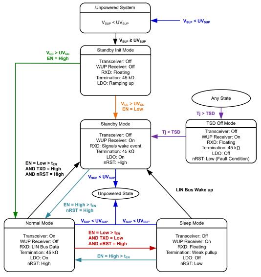
Figure 9-5. Operating State Diagram
