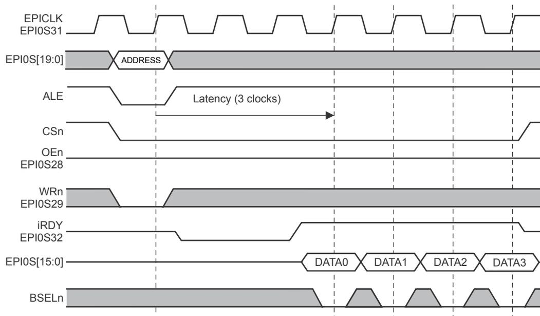
Note that if a read or write transfer attempts to begin during a refresh event, the transfer is held off by the assertion of the iRDY pin by the memory to the EPI module. Figure 11-9 on page 846 and Figure 11-10 on page 847 depict the delay in data transfer during a refresh collision.
