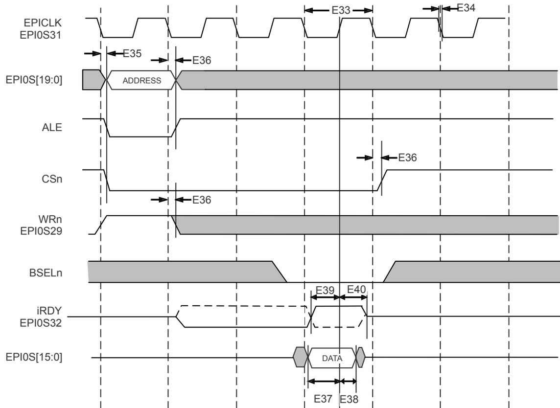
Figure 30-27. PSRAM Single Burst Write
