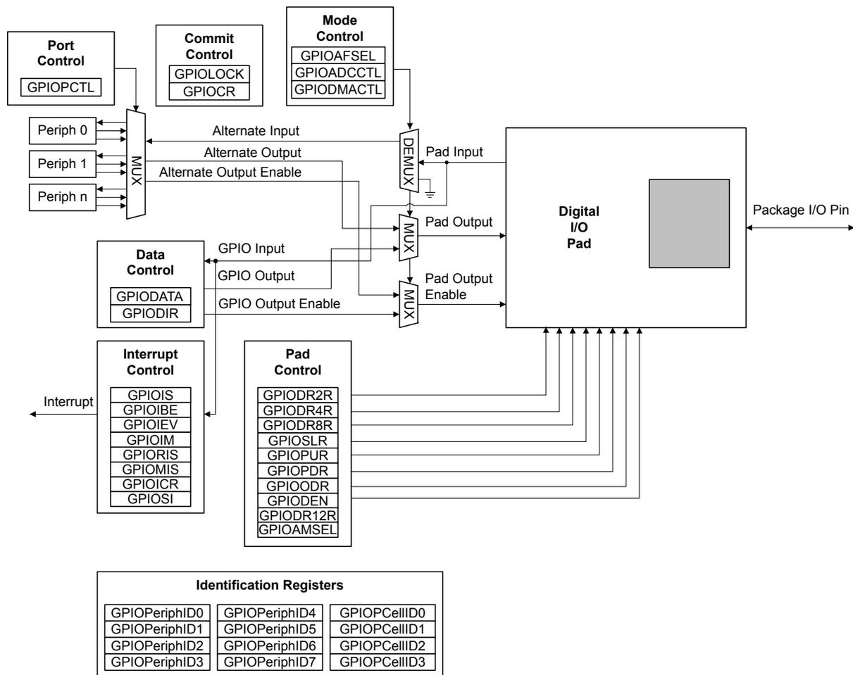
Figure 10-2. Analog/Digital I/O Pads
