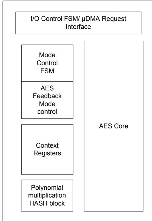
AES is an efficient implementation of the Rijndael cipher (the AES algorithm) and a 128-bit polynomial multiplication (referred to here as GHASH, as per the AES-GCM specification). Rijndael is a block cipher in which each data block is 128 bits. The polynomial multiplication multiplies two 128-bit vectors using the smallest 128-bit irreducible polynomial, represented by the following 128-bit string:  $\{0^{120}\}||10000111$ . The two implementations are combined into the AES wide-bus engine.
