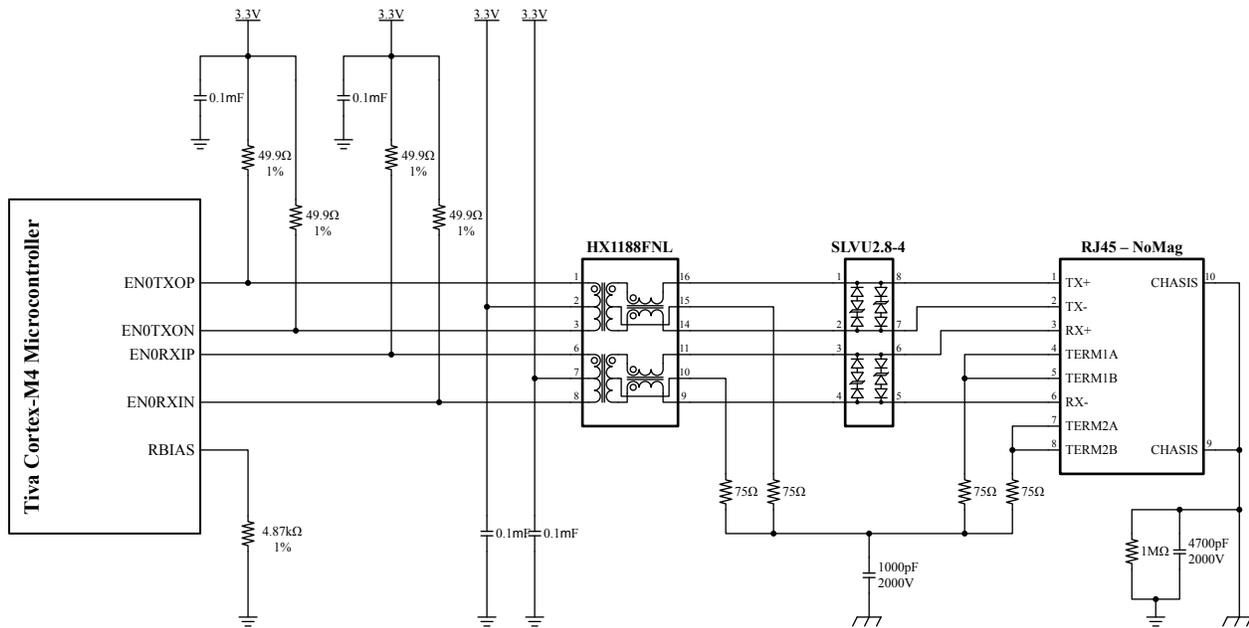
**NOTE:** The 0.1mF capacitors on pins 2 and 7 of the HX1188FNL should be located near the physical pins of the transformer.
