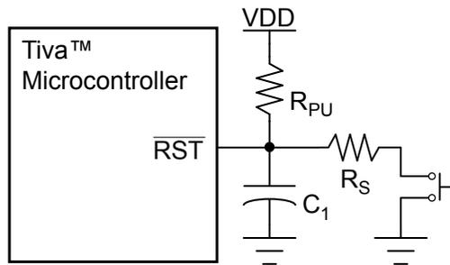
**Note:** Typical  $R_{PU} = 10$  k $\Omega$
