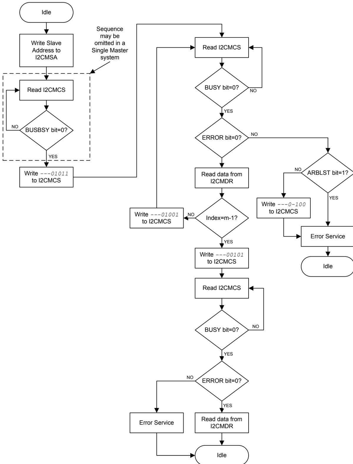
Figure 21-12. Master RECEIVE with Repeated START after Master TRANSMIT
