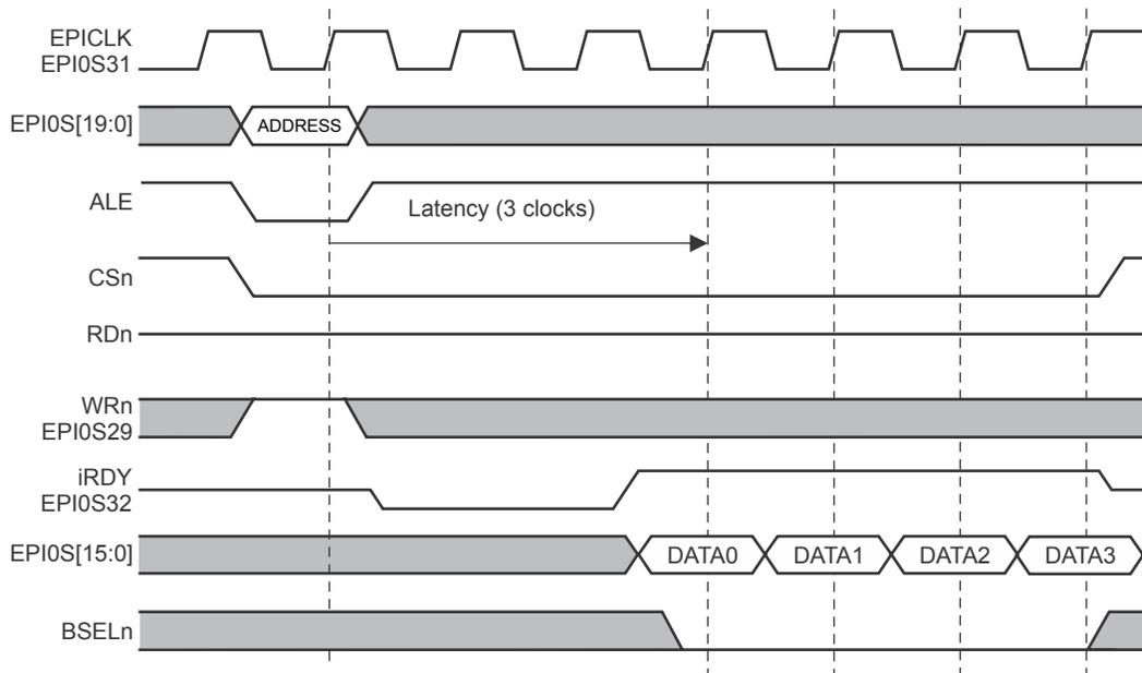
Figure 11-8. PSRAM Burst Write
