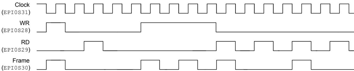
If the `FRMCNT` field is `0x2` and `FRM50` is clear, then the `FRAME` signal pulses high during every third access, and so on for every value of `FRMCNT`, see Figure 11-24 on page 858.
