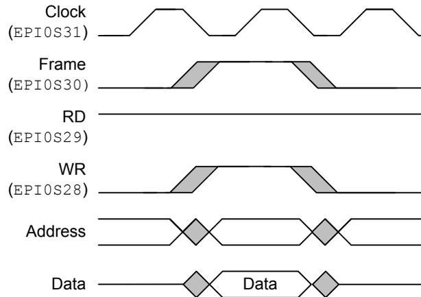
**Figure 11-20. Two-Cycle Read, Write Accesses, FRM50=0, FRMCNT=0, WR2CYC=1**
