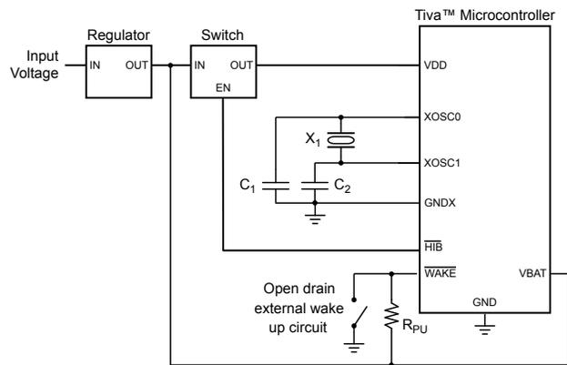
**Note:** Some devices may not supply a `GNDX` signal. See “Signal Tables” on page 1894 for pins specific to your device.
