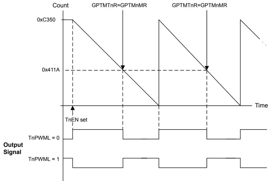
When synchronizing the timers using the **GPTMSYNC** register, the timer must be properly configured to avoid glitches on the CCP outputs. Both the **TnPLO** and the **TnMRSU** bits must be set in the **GPTMTnMR** register. Figure 16-5 on page 1089 shows how the CCP output operates when the **TnPLO** and **TnMRSU** bits are set and the **GPTMTnMATCHR** value is greater than the **GPTMTnILR** value.
