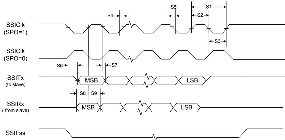
**Figure 30-32. Slave Mode SSI Timing for SPI Frame Format (FRF=00), with SPH=1**
