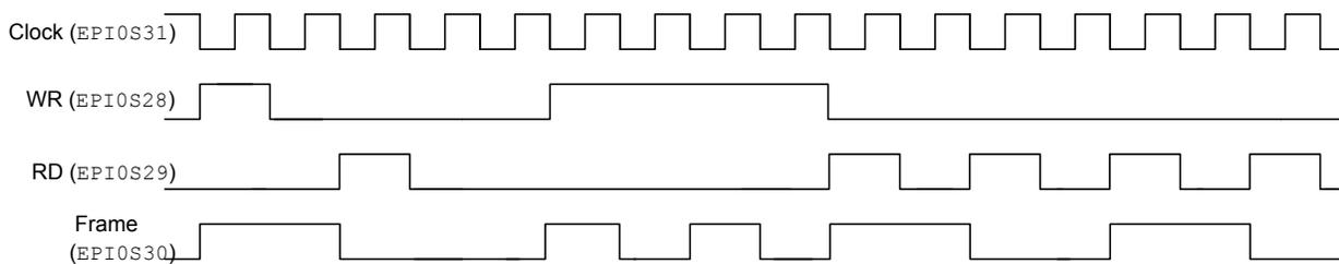
When `FRMCNT=1`, the `FRAME` signal transitions on the rising edge of the `WR` or `RD` strobes for every other access, see Figure 11-26 on page 859.
