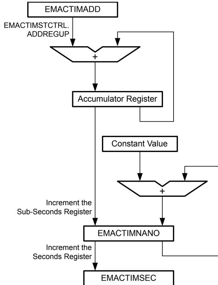
**Note:** The MOSC clock that feeds the PTP reference clock to the System Time Module must be 25 MHz because it is also clocks the integrated PHY module.
