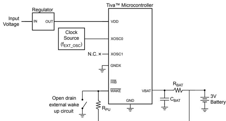
**Note:** Some devices may not supply a GNDX signal. See “Signal Tables” on page 1894 for pins specific to your device.
