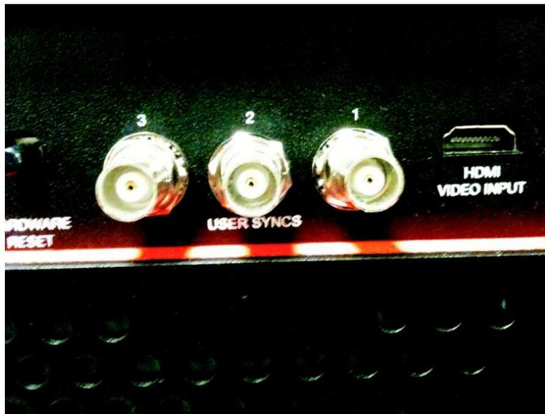
**Figure 5. BNC Connectors for Output Syncs**
