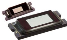
Figure 2-2. 0.2-inch DLP2010 Diagonal DMD compared to a 0.45-inch DLP4501 Diagonal DMD
