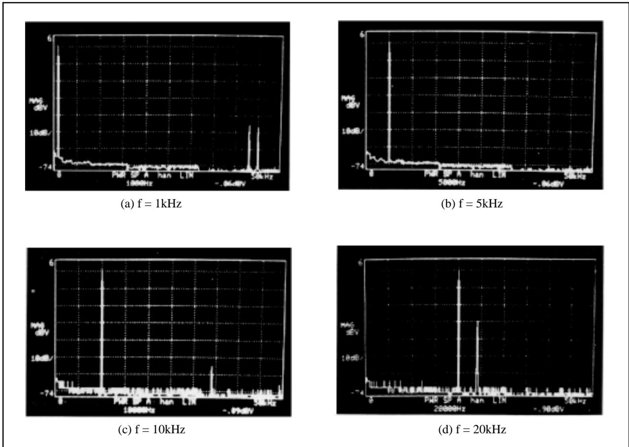
FIGURE 5. Actual Measurement Result of PCM1717 Output Spectrum.
