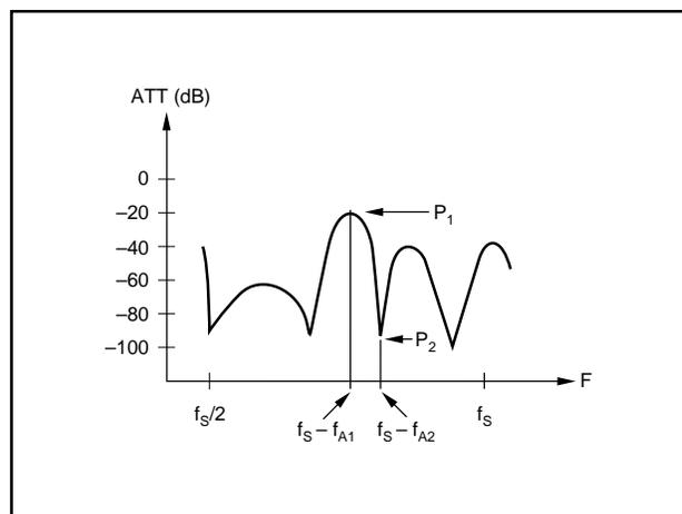
FIGURE 3. Digital Filter Attenuation with Spectrum.
