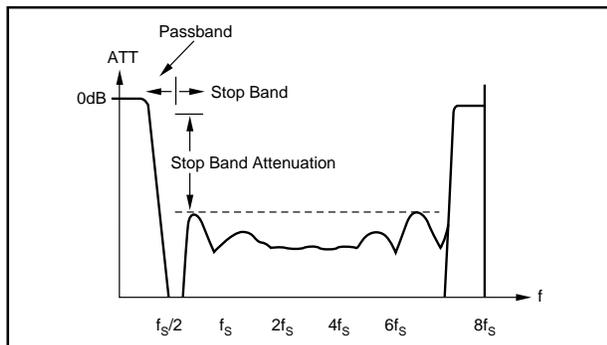
FIGURE 1. Digital Filter Attenuation.
