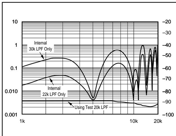
FIGURE 7. THD+N versus Frequency Characteristics with 2nd-Order Post Filter.
