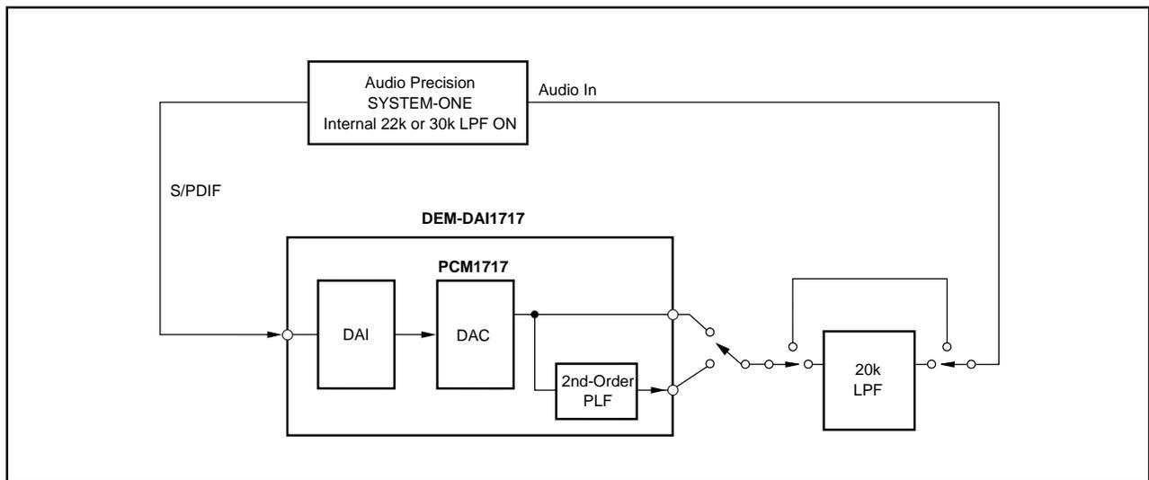
FIGURE 6. THD+N versus Frequency Test Block Diagram.
