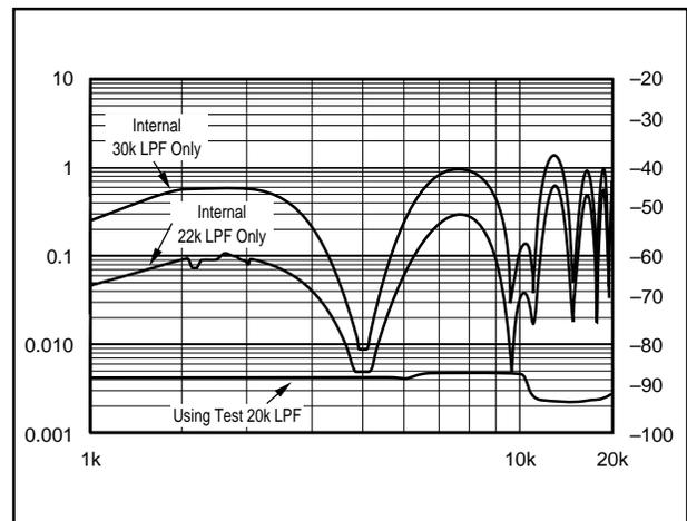
FIGURE 8. THD+N versus Frequency Characteristic without any Post Filter.
