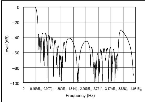
FIGURE 4. Digital Filter Characteristic of PCM1717.
