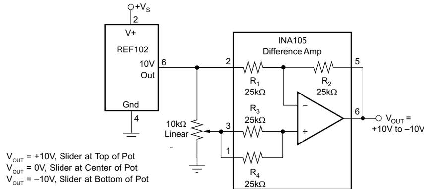
**Figure 2. -10V to +10V Adjustable Precision Voltage Source**
