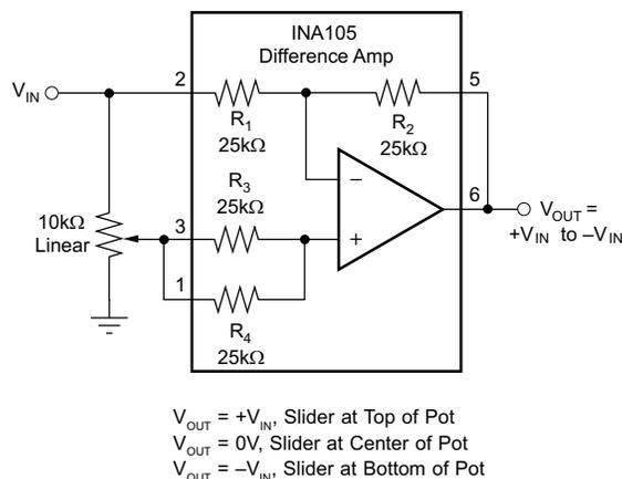
**Figure 1. –1.0V/V to +1.0V/V Linear Gain Control Amplifier**
