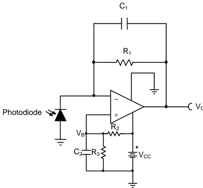
**Figure 2. Typical Photodiode Amplifier Circuit**
