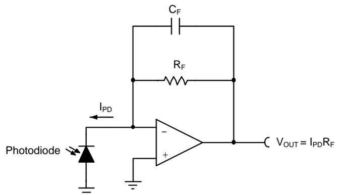
**Figure 1. Typical Transimpedance Amplifier Circuit**
