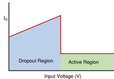
Figure 3. [TPS7A02](#) -  $I_Q$  vs  $V_{IN}$  During Dropout
