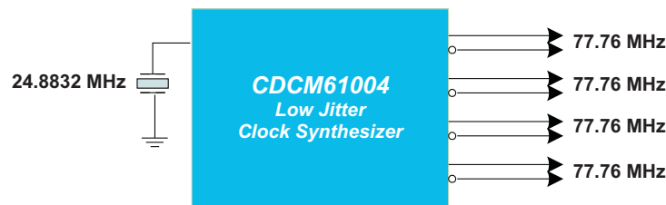
Figure 9. WAN Block Diagram 4
