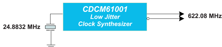
Figure 6. WAN Block Diagram 1
