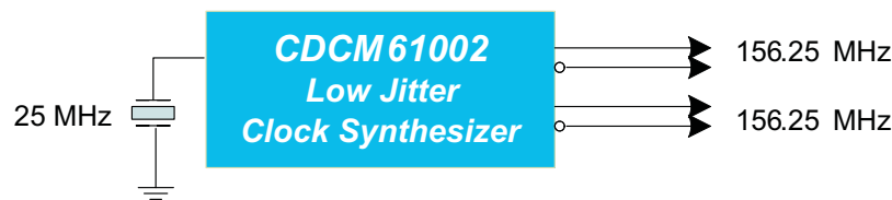
Figure 4. LAN Block Diagram 3
