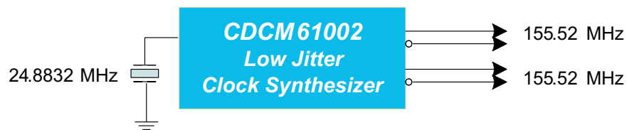
Figure 8. WAN Block Diagram 3
