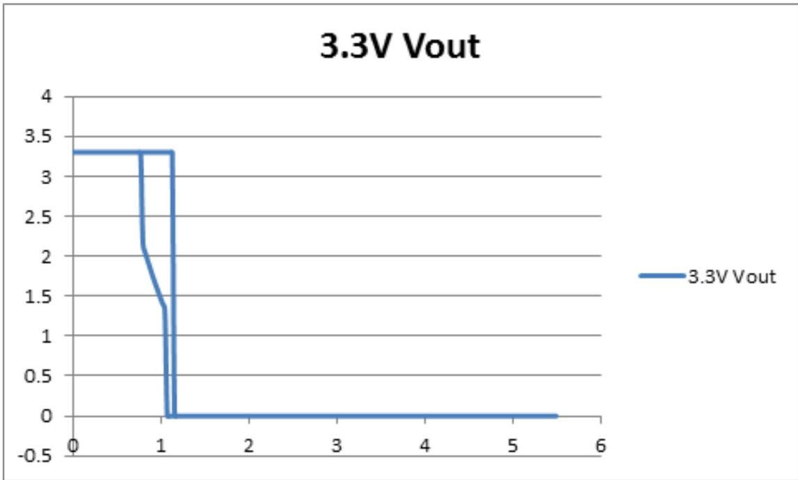
Figure 1. Switching Threshold with 3.3-V Vcc
