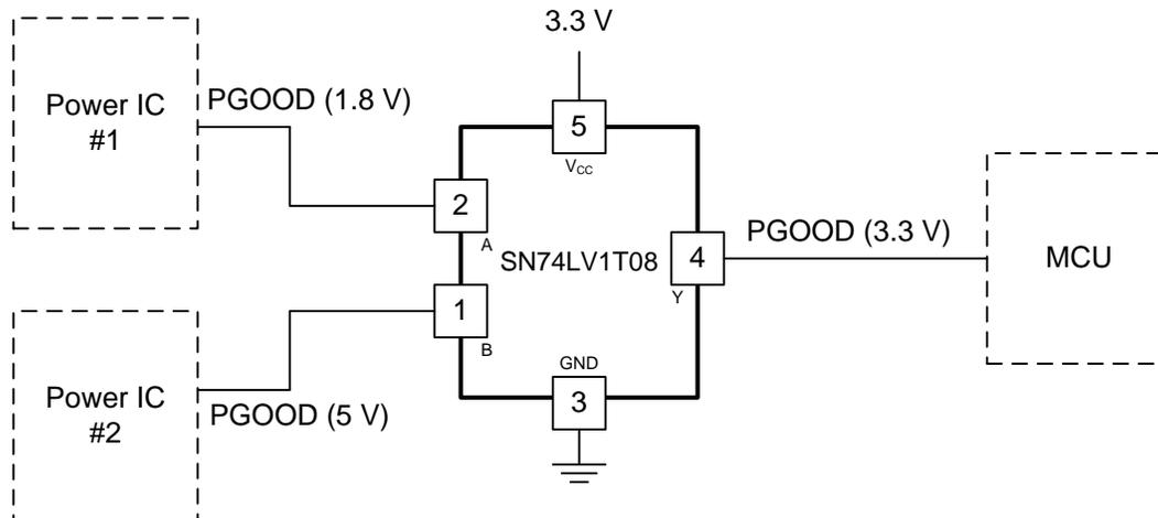
Figure 4. PGOOD Circuit with LV1T Acting as Several Devices
