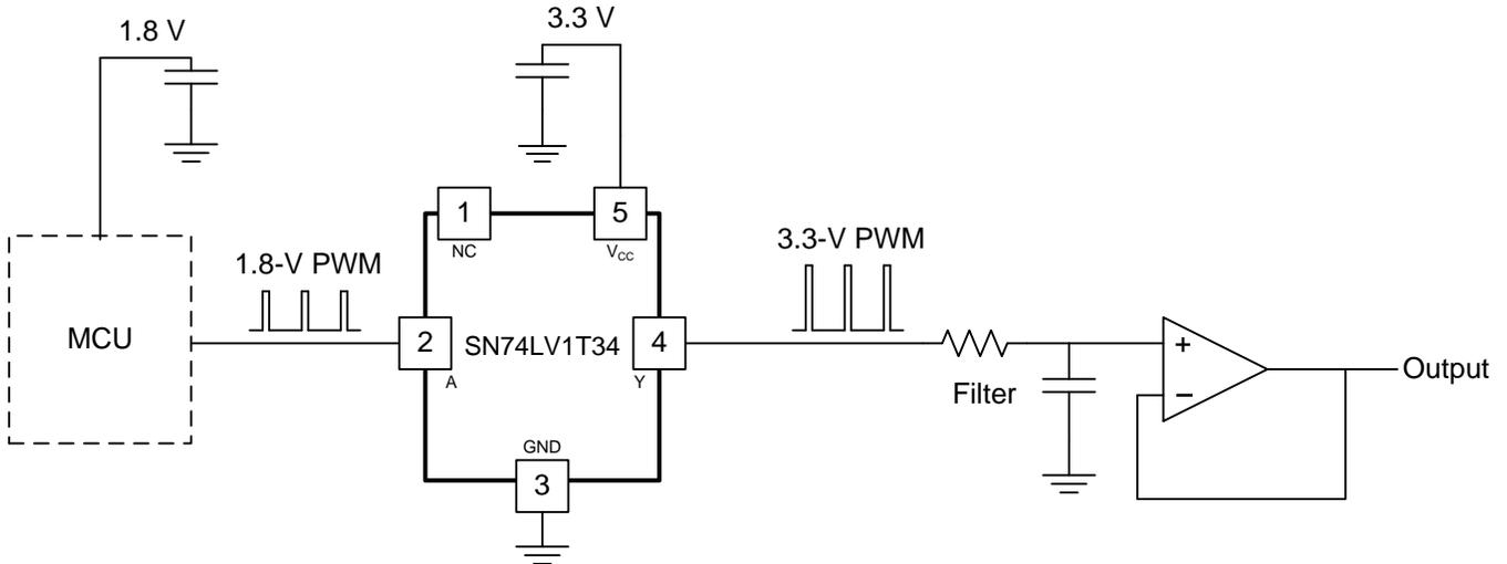
**Figure 3. Example Schematic for LV1T PWM Circuit**
