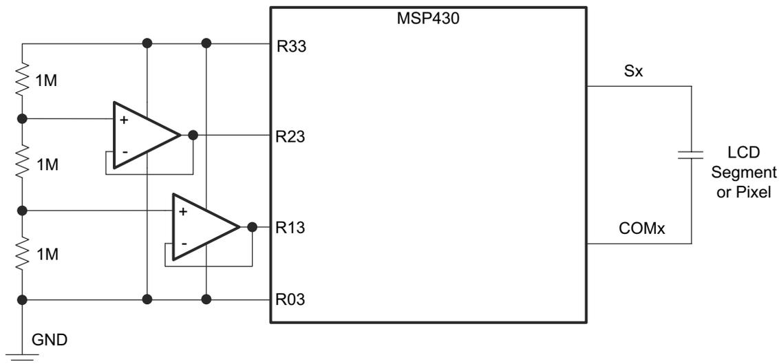
**Figure 3. Using Opamps to Buffer Node Voltages**
