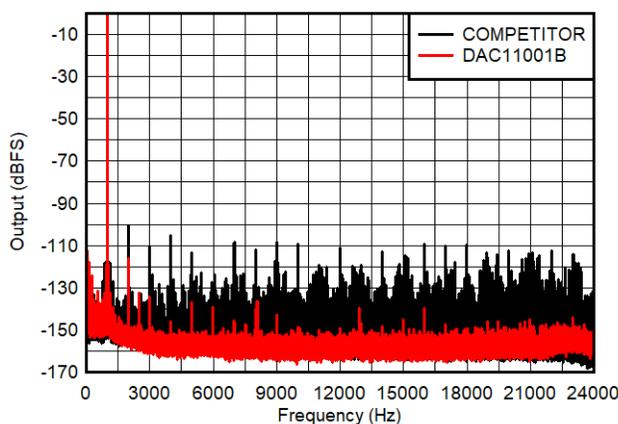
**Figure 4-1. Spectrum DAC11001B vs Competitor – 1 kHz, 10 kSPS Update Rate, 9Vpp**
