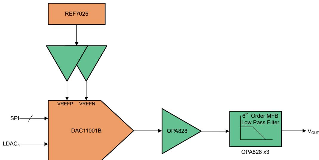
**Figure 3-1. DAC11001B Signal Chain Block Diagram With Companion Parts**
